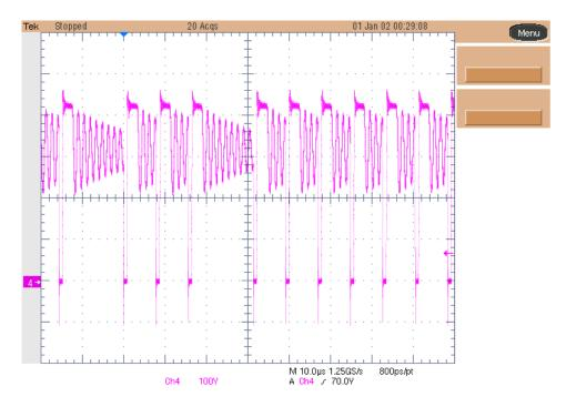
Ch4: Drain voltage (100V/div, 100usec/div, No BWL). Vin = 320Vdc, Iout=30mA
