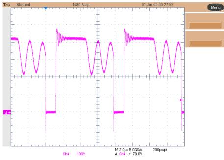
By reducing the load, the converter enters the pulse skipping mode, as shown in the picture below.
