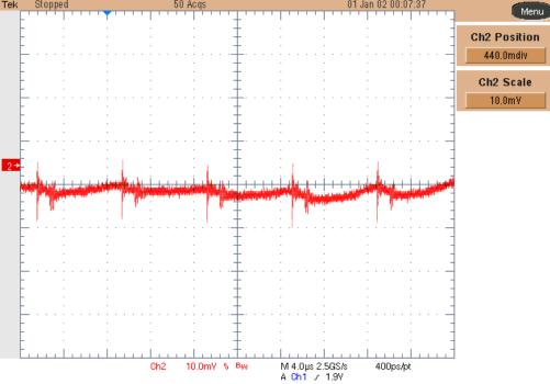
The picture below shows how the output ripple voltage is increased during a burst mode condition. The input was unmodified and the output set to 30mA.
