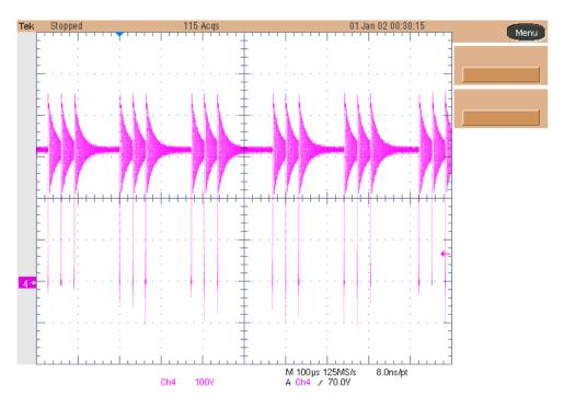
Ch4: Drain voltage (100V/div, 200usec/div, No BWL). Vin = 320Vdc, No Load
