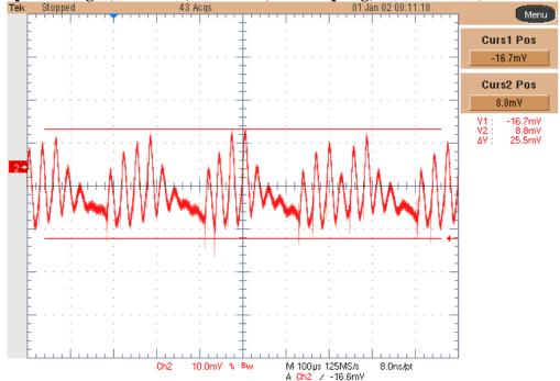
Ch.2: Output Voltage (10mV/div, 100us/div, AC coupling, 20MHz BWL)
