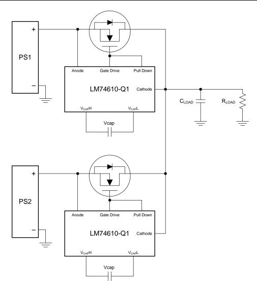
Figure 1. LM74610-Q1 Typical OR-ing Application Circuit
