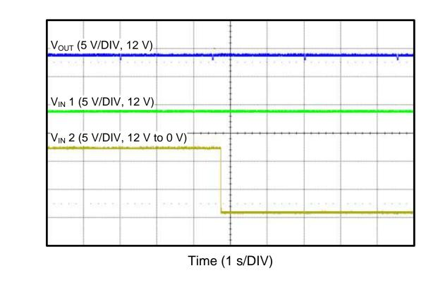
Figure 9. LM74610-Q1 OR-ing Waveform
