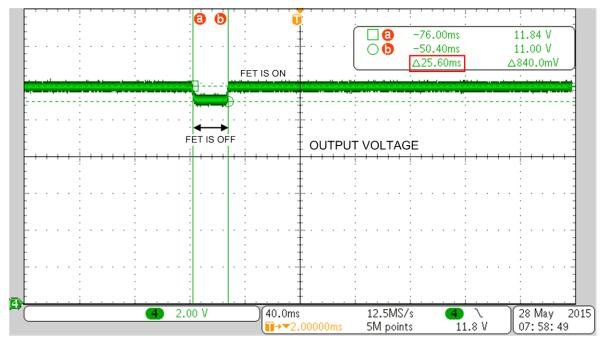
Figure 5. Periodic Body Diode Voltage Drop at the Output
