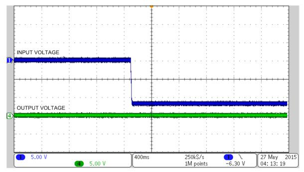
Figure 4. Response to Start Up Reverse Polarity
