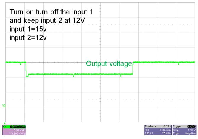
Figure 7. OR-ing Application Output Voltage Waveform
