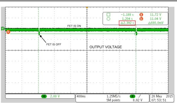
Figure 6. The LM74610-DQEVM Output Voltage Waveform
