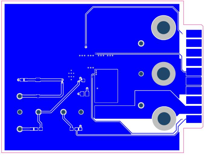
Figure 7. Bottom Layer Routing
