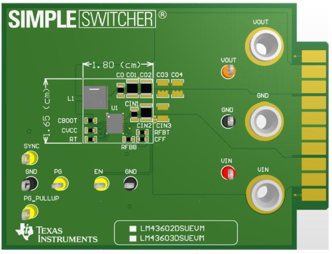
Figure 1. Top View of LM43603DSUEVM
