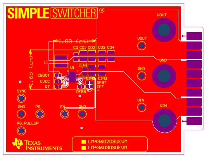
Figure 3. Top Assembly Layer
