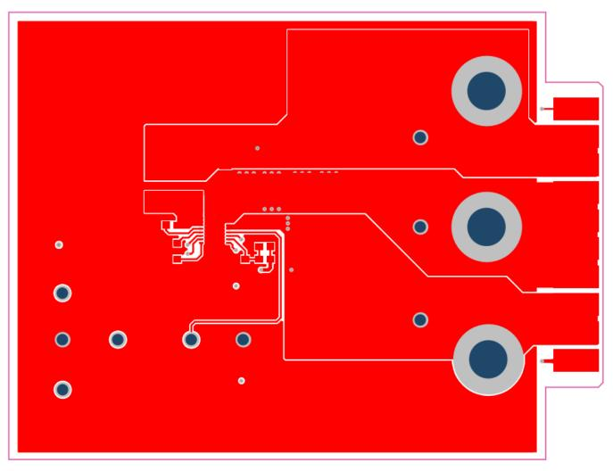
Figure 4. Top Layer Routing
