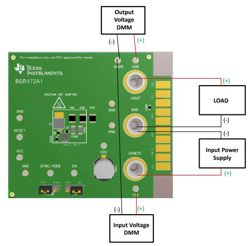
Figure 1-1. EVM Board Connections
