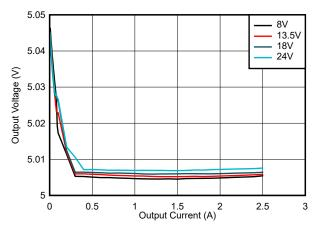
Figure 3-1. Efficiency: AUTO Mode, V<sub>OUT</sub> = 5 V, f<sub>SW</sub> Figure 3-2. Line and Load Regulation: AUTO Mode, V<sub>OUT</sub> = 5 V, f<sub>SW</sub> = 2100 kHz
