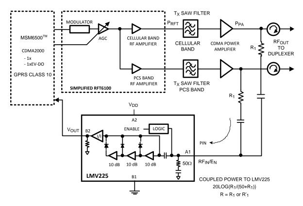
Figure 8. Dual-Band CDMA2000 Transmit Architecture
