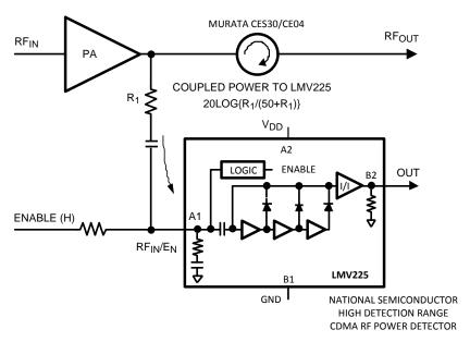
Figure 2. Transmit Radio Architecture
