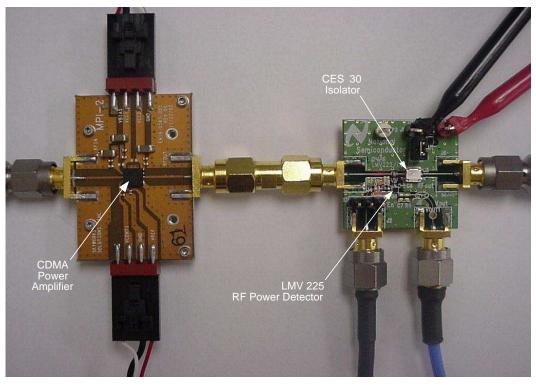
Figure 4. LMV225 Eval Board + CDMA PA's Module
