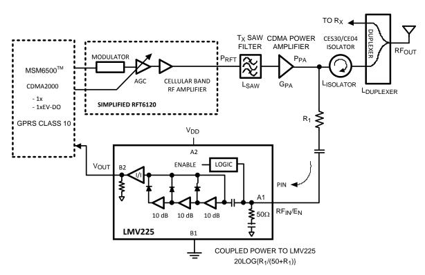
Figure 5. Single-Band CDMA2000 T<sub>x</sub> Architecture
