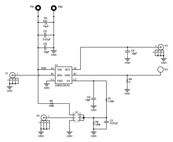
Figure 3. Evaluation Board Schematic
