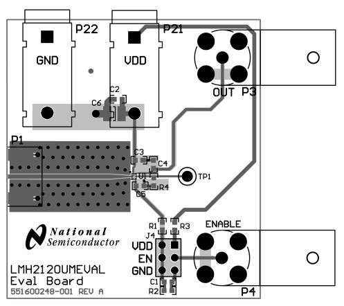
Figure 5. Board Layout of Evaluation Board
