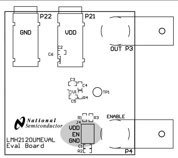
**Figure 2. Jumper Positions**
