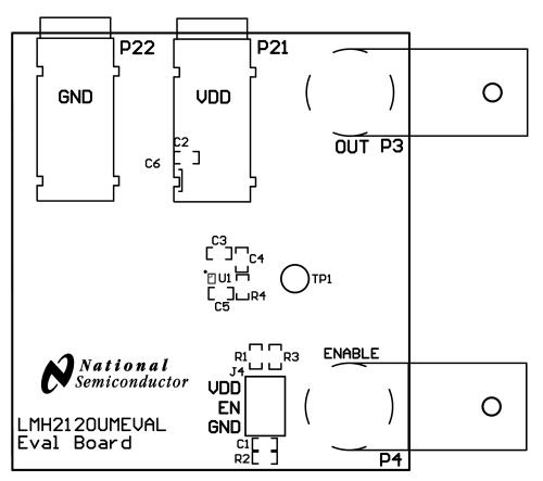
Figure 4. Component Locations of Evaluation Board
