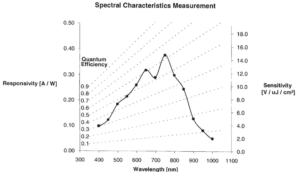
Figure 5. Spectral Characteristics for the Visible and Near IR Wavelengths
