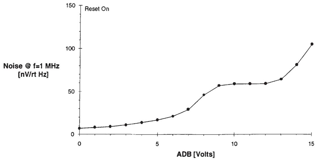
Figure 19. Noise-Power Spectral Density Measured at  $f = 1$  MHz with Reset On, as a Function of the Amplifier Supply Voltage
