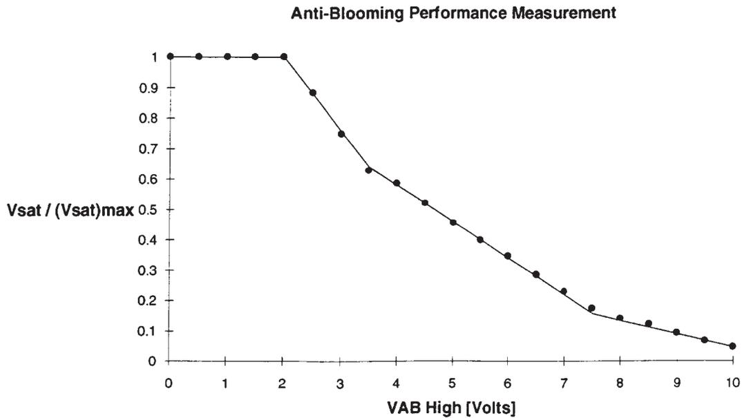
Figure 7. Saturation Voltage as a Function of the Antiblooming High Level
