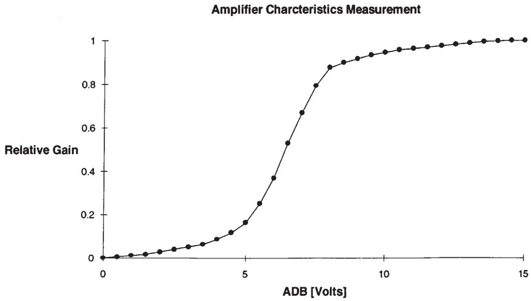
Figure 13. Amplifier Gain Measured Using the Reset Feed Through
