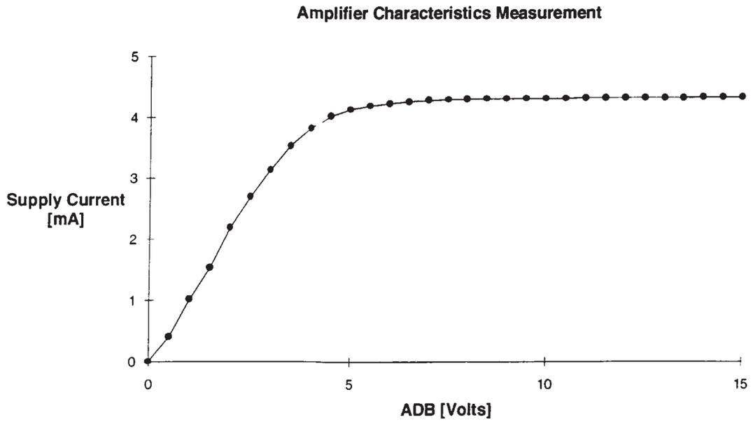
Figure 10. Amplifier Supply Current as a Function of the Supply Voltage
