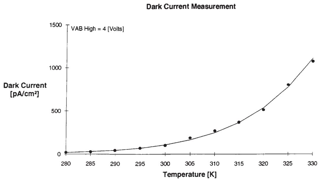
Figure 2. Dark Current as a Function of Temperature
