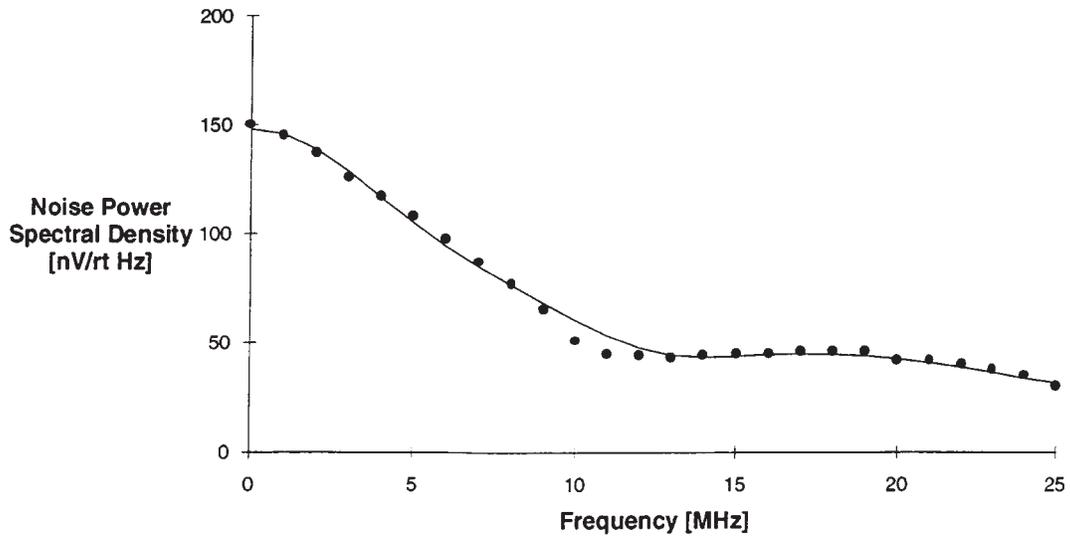
Figure 18. Noise-Power Spectral Density, Measured for  $\tau = 150 \text{ ns}$ ,
