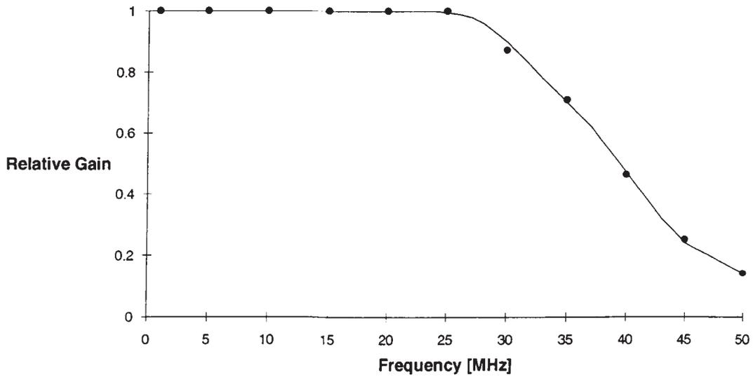
Figure 12. Amplifier Frequency Response Measured Using the Reset Feed Through
