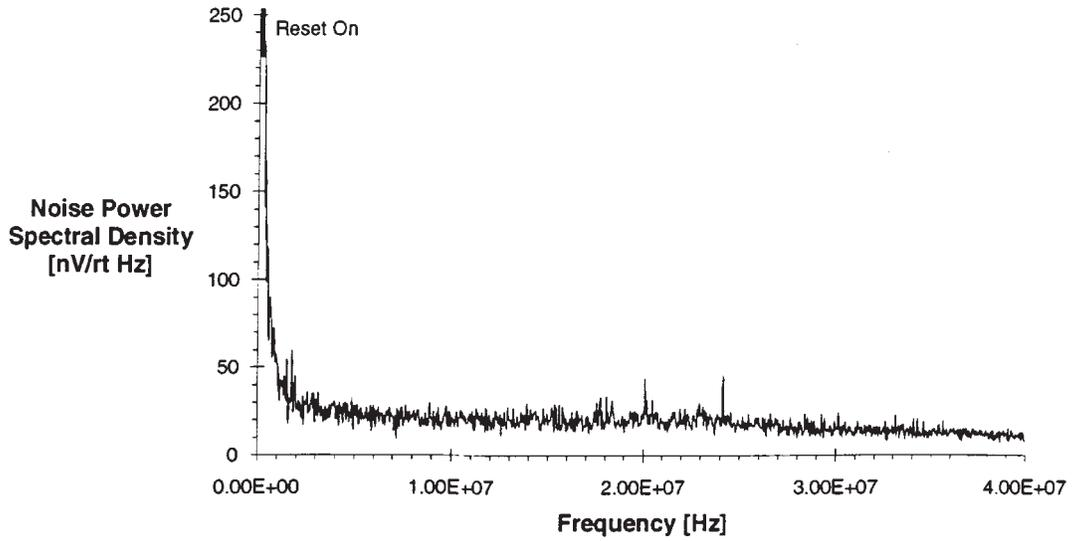
Figure 17. Noise-Power Spectral Density Measured With Reset On
