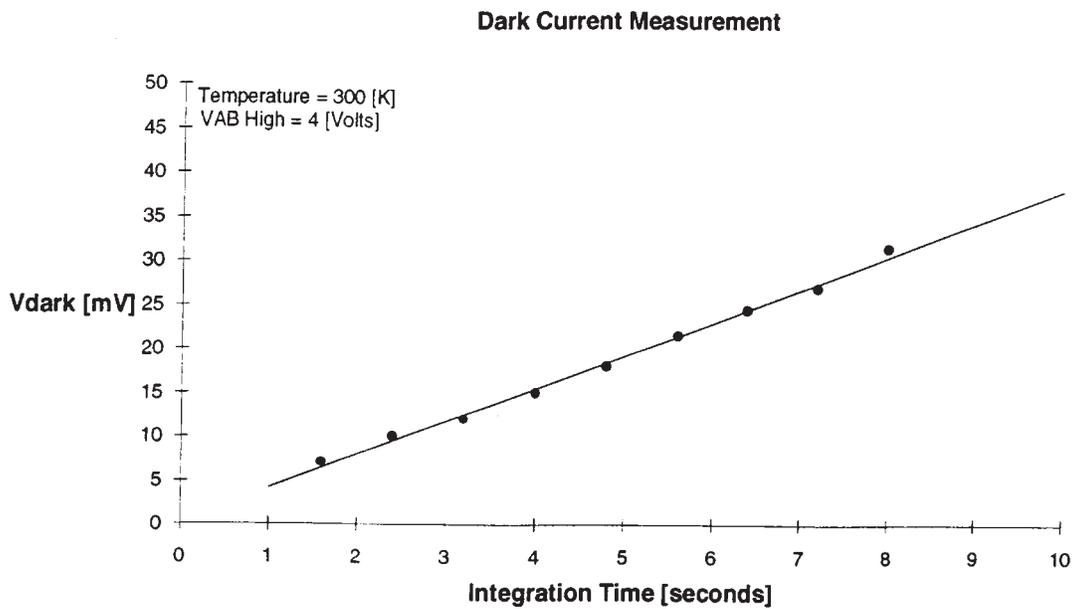
Figure 1. Measured Dark Voltage at the Device Output as a Function of Integration Time Under Normal Operating Conditions
