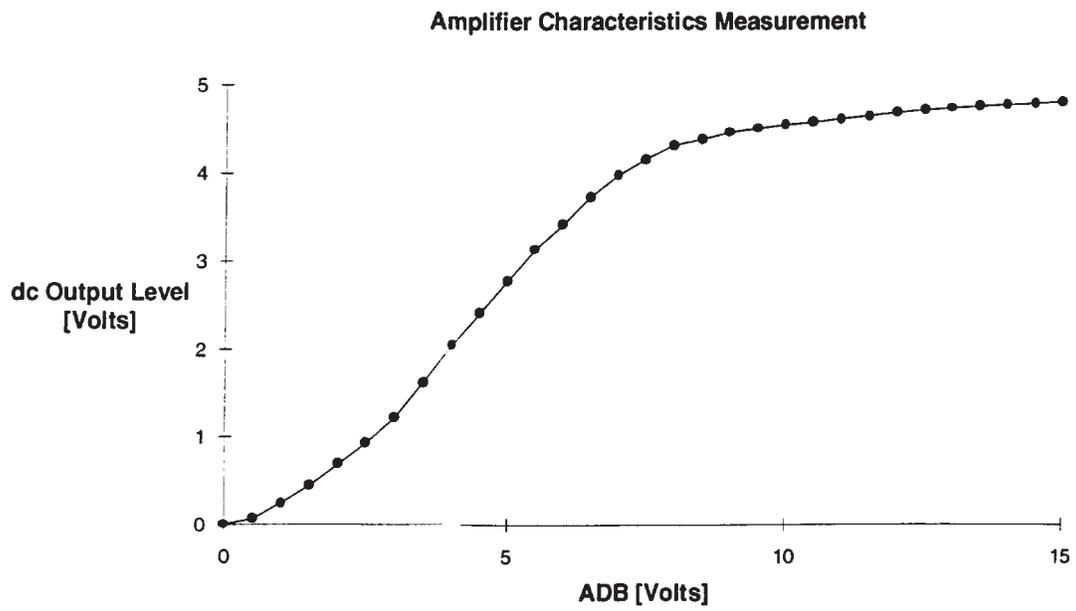
Figure 9. Amplifier Output dc Level as a Function of the Supply Voltage
