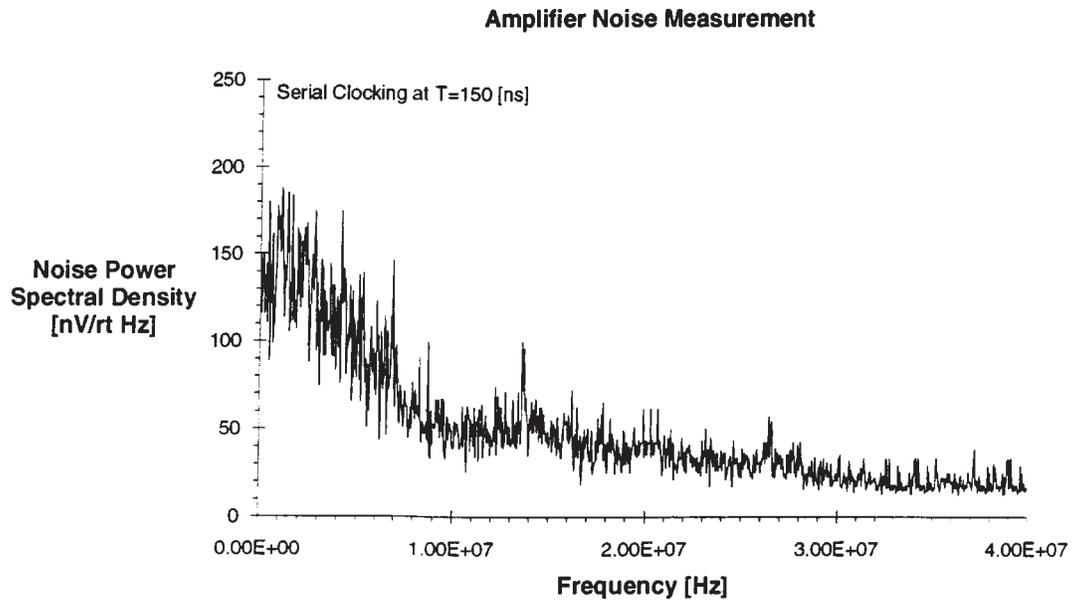
Figure 16. Noise-Power Spectral Density Measured at the Normal Serial-Clocking Speed
