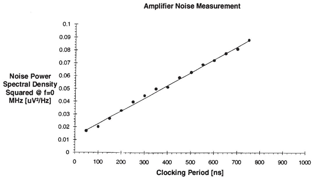
Figure 15. Squared Noise-Power Spectral Density Measured at  $f = 0$  as a Function of the Reset Period
