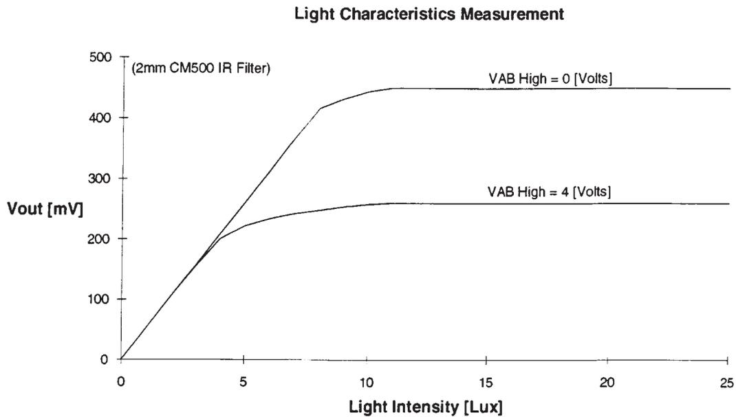
Figure 6. Measured Sensor Output as a Function of Light Intensity
