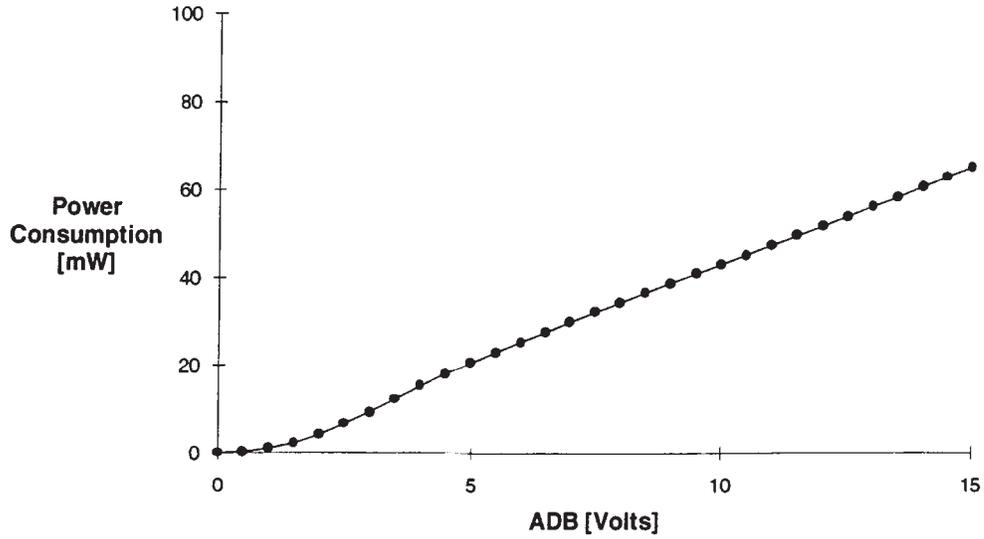
Figure 11. Power Consumption as a Function of the Supply Voltage
