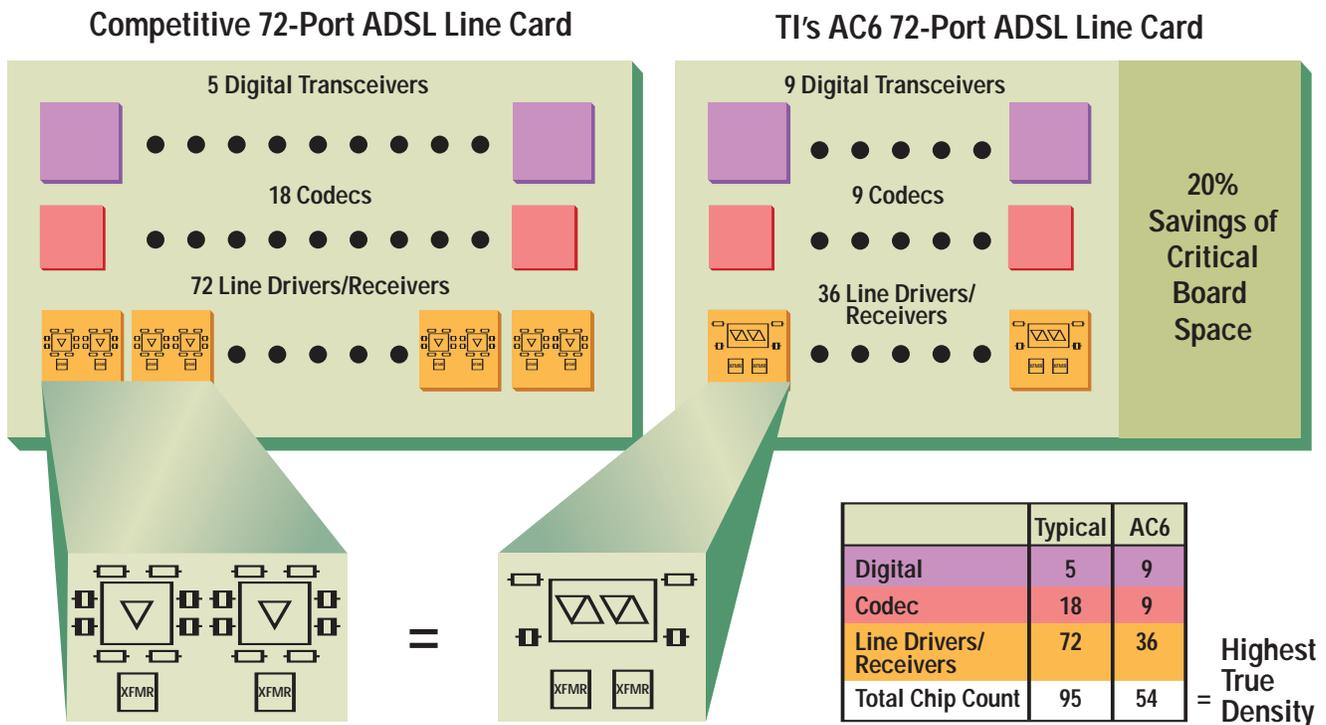
AC6 provides the industry's highest "true" density against 16-port configuration competitive offerings. True density is defined as the combination of total number of channels the chipset supports, the power-consumption of the board and the board area per port.
