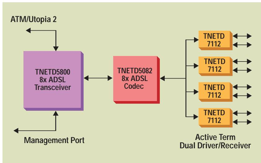
The three-chip AC6 includes an octal transceiver, codec and dual-line drivers.
