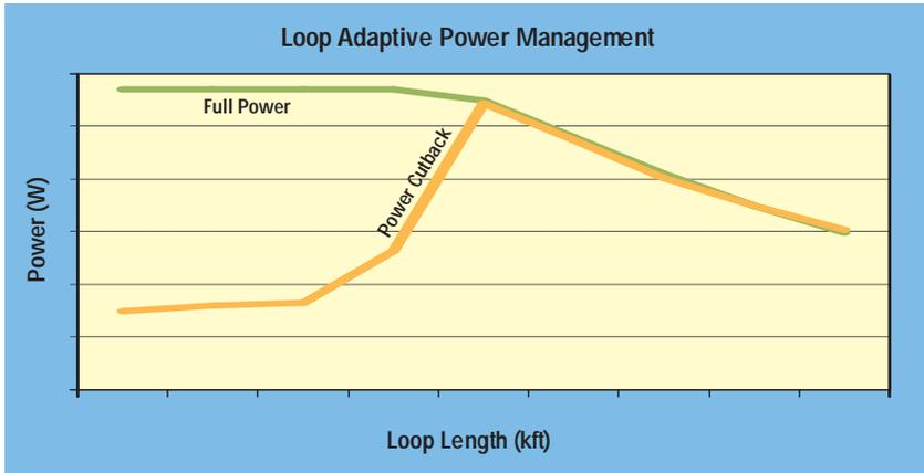
AC6's loop adaptive feature allows you to control power based on varying throughput at different loop lengths. Service providers can now optimize every system or line card at certain data rates or power budgets.
