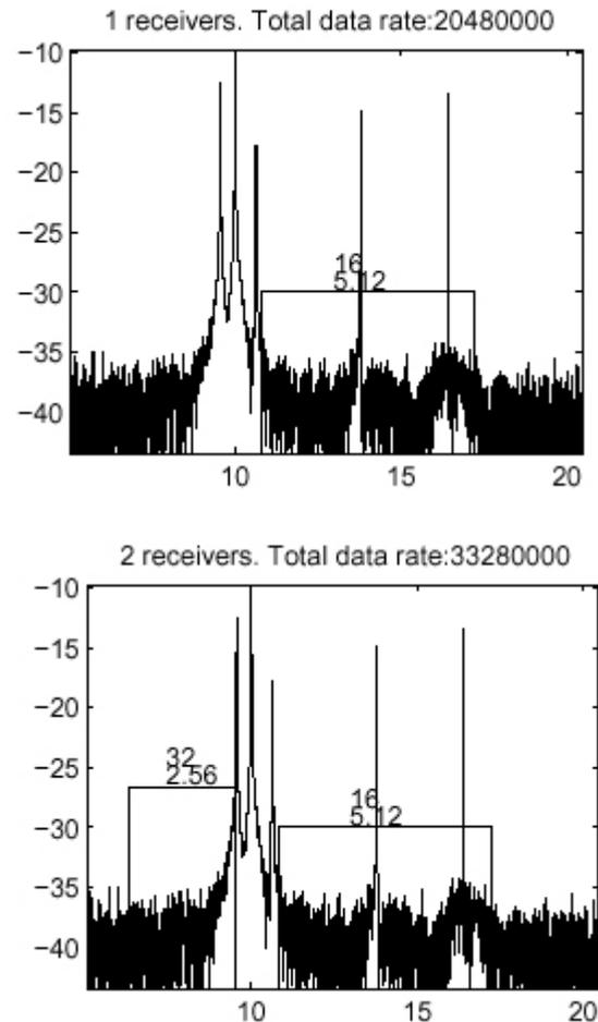
**Figure 2: DUCA Channel Spectrum with one and two receivers**
