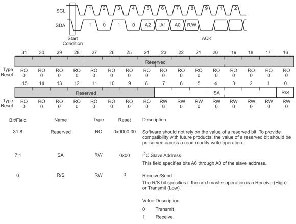
Figure 7. I2CMSA and Slave Address Representation
