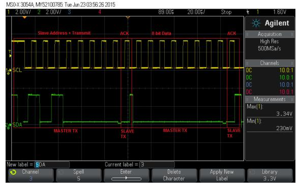
Figure 4. Data Frame Write
