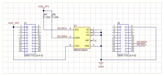
Figure 6. Circuit Schematic
