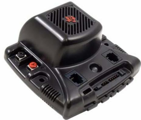
Figure 1. Brushed DC Motor Control Module
