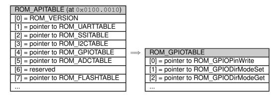
From this, the address of the ROM\_GPIOTABLE table is located in the memory location at  $0 \times 0100.0020$ . The address of the ROM\_GPIODirModeSet() function is contained at offset  $0 \times 4$  from that table. In the function documentation, this is represented as:
