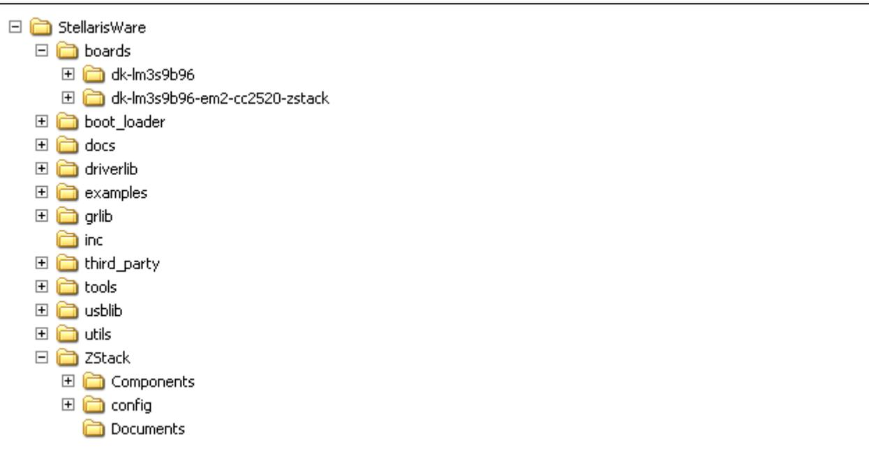
**Directory structure after installation of StellarisWare for DK-LM3S9B96 and the EM2/ZigBee support package**
