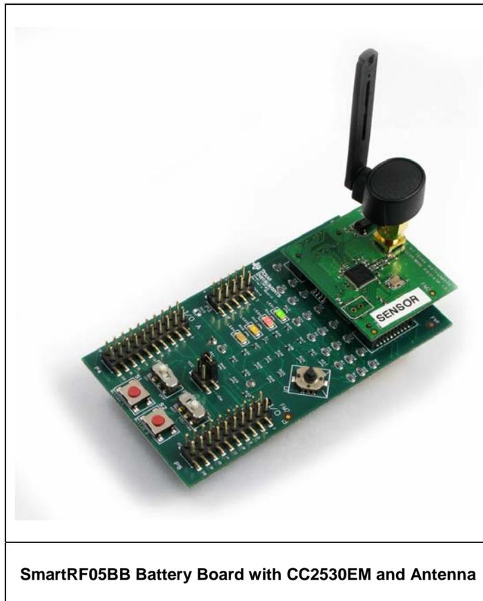
The Stellaris 2.4 GHz ZigBee Wireless Kit includes two SmartRF05BB battery boards, two CC2530EM ZigBee modules, and antennas. Do the following to set up the boards:
