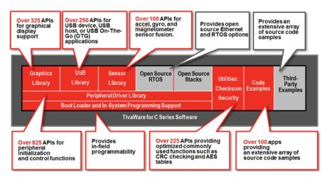
Figure 5: TI's TivaWare™ software provides a comprehensive variety of APIs to significantly simplify development of core product features.
