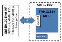
Figure 3: A traditional Ethernet link (a) requires an external PHY, numerous passives, and other components. By integrating the PHY, (b) TM4C129x MCUs reduce a system's board space needs, energy consumption and cost.
