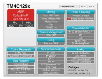
Figure 2: The TM4C129x MCUs are the industry's first ARM<sup>®</sup> Cortex<sup>®</sup>-M4 MCU with an integrated 10/100 MAC+PHY. With their extensive capabilities, they are ideal for implementing both simple and embedded control IoT gateways.
