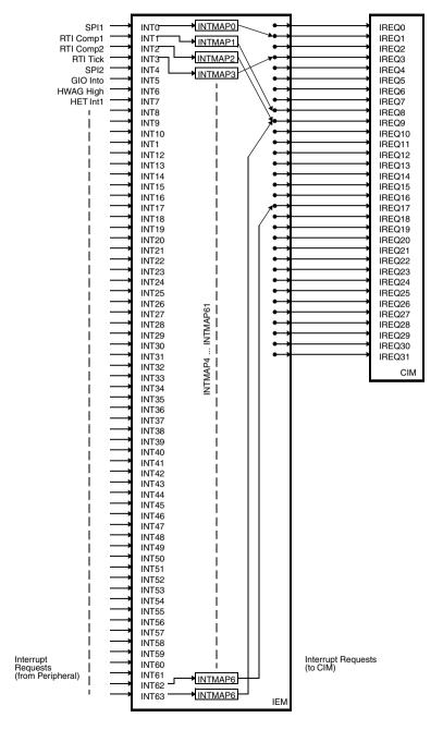
As illustrated in Figure 1, the IEM is used to map the interrupt requests from peripheral modules in the 470R1Vx system (INT[63:0]) to the CIM interrupt requests IREQ[31:0].
