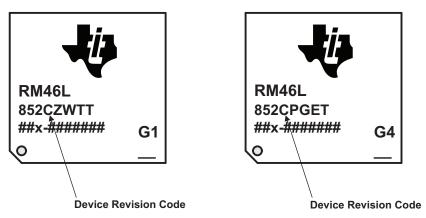
Figure 1. Device Revision Code Identification
