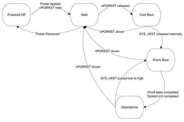
Figure 6. Operating States of the Hercules MCU
