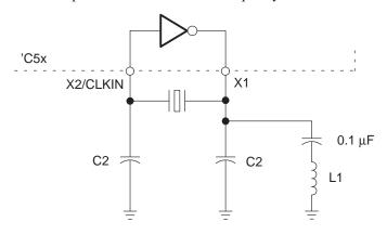
Figure 16. Oscillator Circuit for Overtone Crystal Operation
