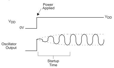
Figure 18. Oscillator Startup
