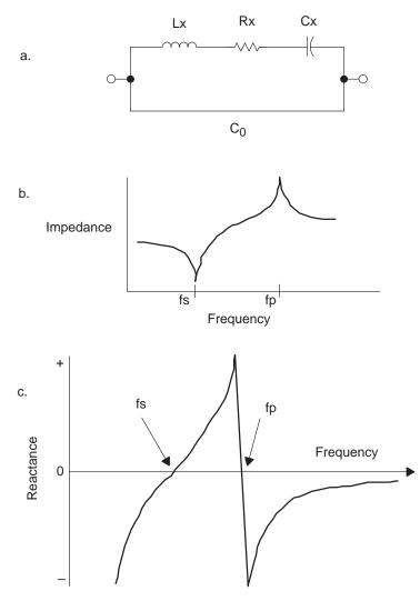
Figure 2. Crystal Equivalent Circuit Model
