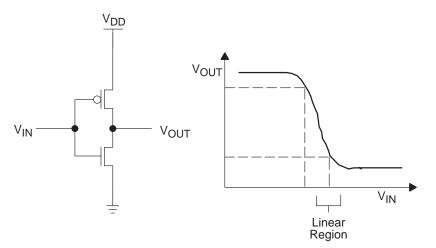
Figure 8. Digital Inverter Circuit and Its Transfer Characteristic
