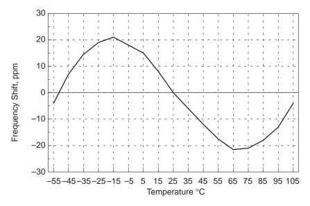
Figure 19. Example Frequency-Temperature Characteristic of AT-Cut Crystals
