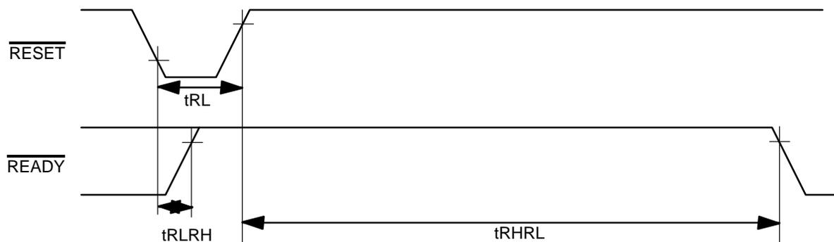
Table B–3. Reset Timing ( $V_{DD} = 1.8\text{ V to }3.3\text{ V}$ ,  $T_A = 0^\circ\text{ C to }70^\circ\text{ C}$ )
