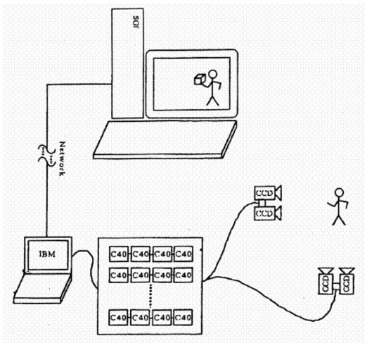
Note: From right to left: The cameras, TMS320C40 parallel DSP, machine, and client.
