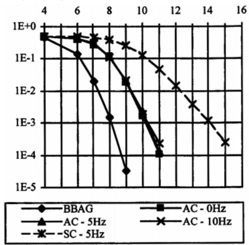
Figure 10. BER=f(SNR in dB) for a Channel with 2 Paths
