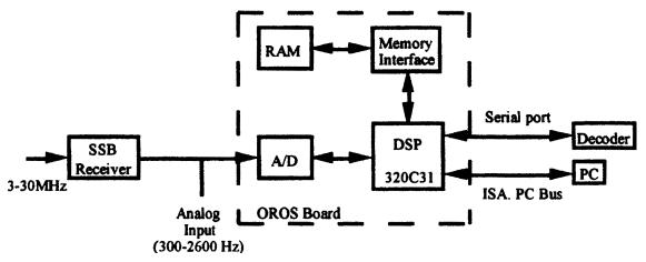
To test the MODEM transmitter, random data is sent from the DSP through the ISA PC bus. Handled data files are sent back to the PC. The DSP output data is converted from digital to analog and the analog output is then used to test the transmission. The data is subsequently up-converted and sent through the ionospheric channel.
