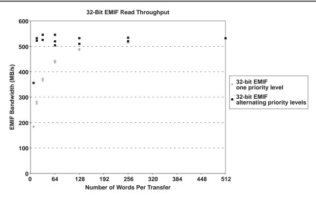
Figure 6. Read Throughput for Multiple 2-D EDMA Transfers from a 133-MHz, 32-bit EMIF
