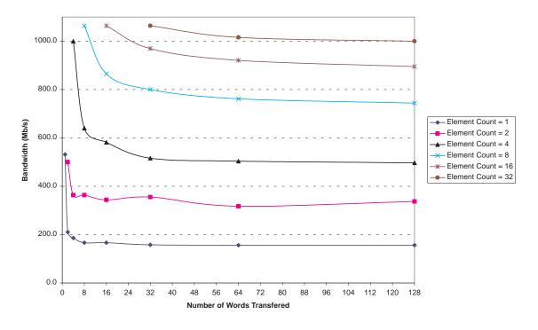
64-Bit EMIF 2D Write Transfer Bandwidth for Various Element Counts
