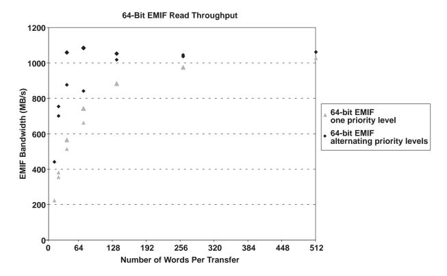
Figure 7. Read Throughput for Multiple 2-D EDMA Transfers from a 133-MHz, 64-bit EMIF
