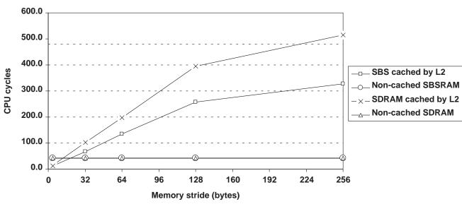
Average CPU Cycles per STW 600 MHz C64x writing to 64-bit, 133-MHz SBSRAM and SDRAM
