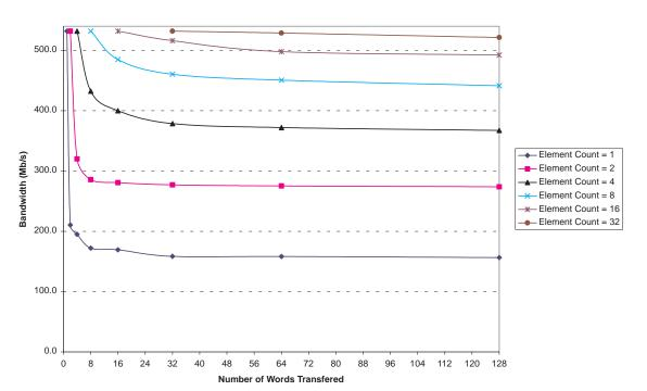
32-Bit EMIF 2D Write Transfer Bandwidth for Various Element Counts
