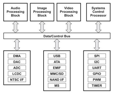
Figure 1. SoC Block Diagram
