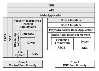
Figure 6. Software Architecture
