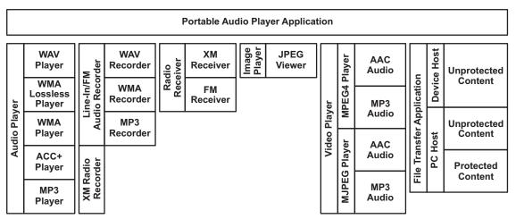
The audio system on a portable device has to handle the digital rights management (DRM) for media files to protect copyrights, allow connectivity to a personal computer (PC) for download and/or upload of files, connectivity between two devices, compressed audio (MP3, AAC, ...) file playback, FM and/or satellite radio reception, and recording of microphone and/or radio content in compressed form.
