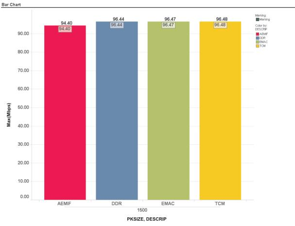
Figure 28. Effect of Descriptor Memory Location on the EMAC Throughput for 100 Mbps Mode
