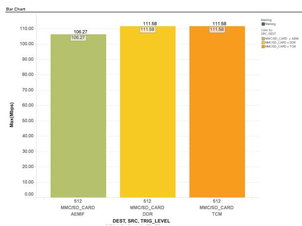
Figure 36. Throughput for MMC/SD Read
