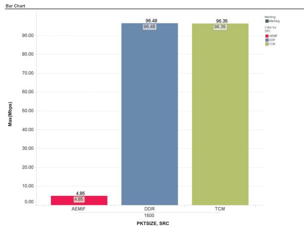
Figure 29. Effect of Source Memory Location on the EMAC Throughput for 100 Mbps Mode
