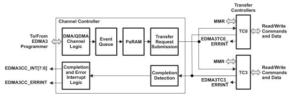
Figure 7. EDMA3 Controller Block Diagram
