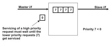
Figure 5. Bridge Head of Line Blocking
