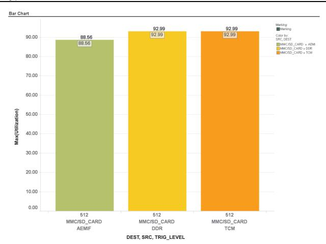
Figure 34. Percentage Utilization for MMC/SD Read
