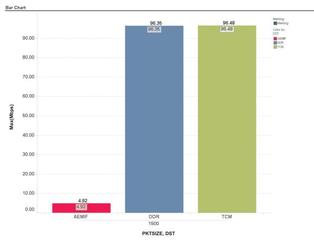
Figure 30. Effect of Destination Memory Location on the EMAC Throughput for 100 Mbps Mode
