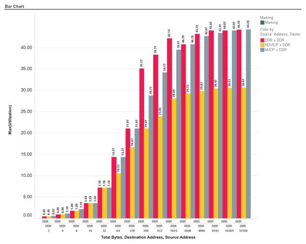
Figure 12. Utilization of EDMA for HDVICP, MJCP to DDR Access
