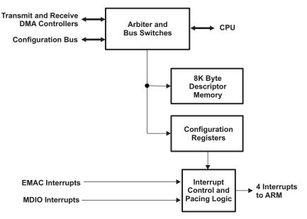
Figure 23. EMAC Control Module Block Diagram
