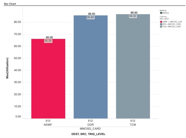
Figure 35. Throughput for MMC/SD Write
