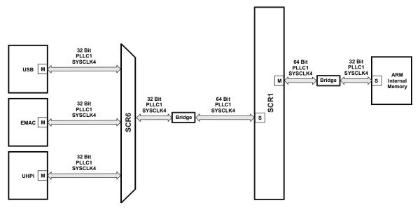
Figure 4. Bus-Width and Clock Rate Conversion
