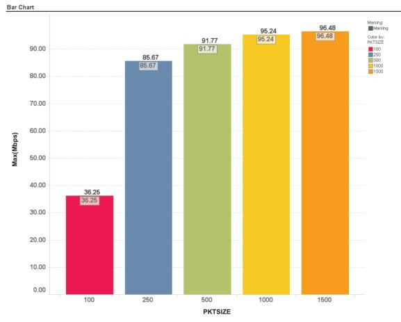
Figure 27. Effect of Packet Size on the EMAC Throughput for 100 Mbps Mode
