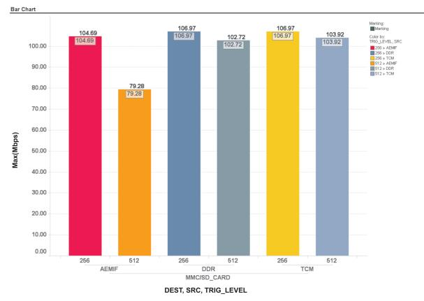
Figure 37. Throughput for MMC/SD Write With Different FIFO Trigger Levels
