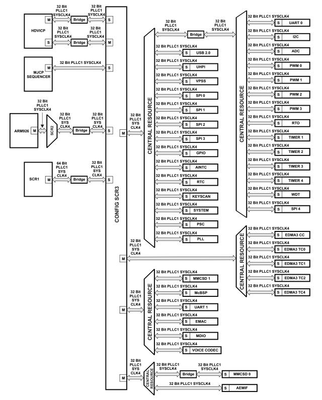
Figure 2. TMS320DM36X Peripheral Configuration Bus
