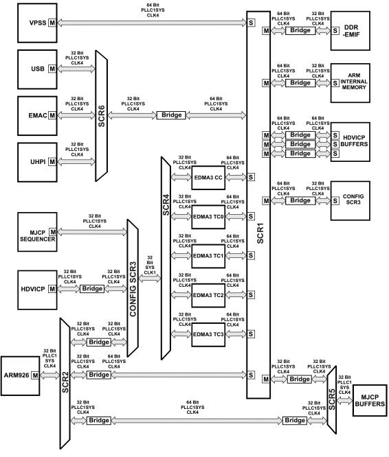
Figure 1. TMS320DM36x System Interconnect Block Diagram
