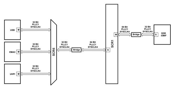
Figure 6. EMAC-to-DDR Transfer
