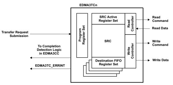
Figure 9. EDMA3 Transfer Controller (EDMA3TC) Block Diagram
