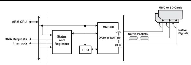
Figure 32. MMC/SD Card Controller Block Diagram
