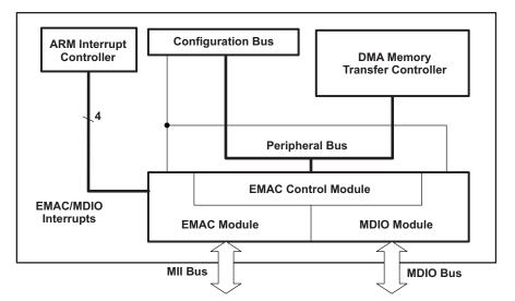
Figure 22. EMAC and MDIO Block Diagram
