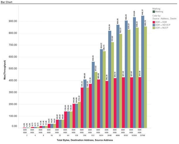
Figure 10. Throughput of EDMA for DDR to HDVICP, MJCP and DDR Access
