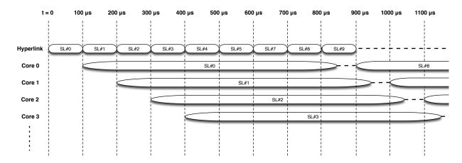
Figure 10. Example timing diagram for input data streaming into MSMC SRAM of a DSP in case one scanline is acquired every 100 μs and assuming that it takes 740 μs for each core to beamform a scanline. Each core starts processing the scanline assigned to it after all the data for that scanline are transferred into MSMC SRAM. In this diagram, it is assumed that data are brought from ADCs into C6678's MSMC SRAM via Hyperlink.
