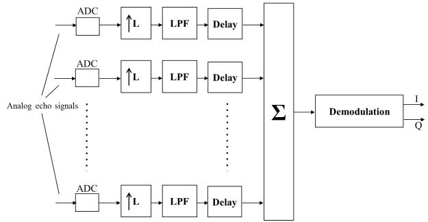
Figure 3. Interpolation beamforming (IBF) block diagram. L is the upsampling ratio.
