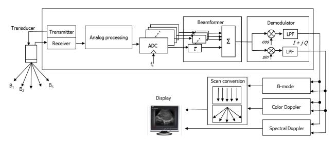
Figure 1. Block diagram of a medical ultrasound machine.
