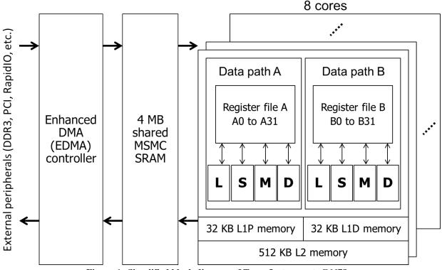
Figure 4. Simplified block diagram of Texas Instruments C6678.
