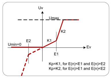
Figure 10. Non-Linear Control of PFC
