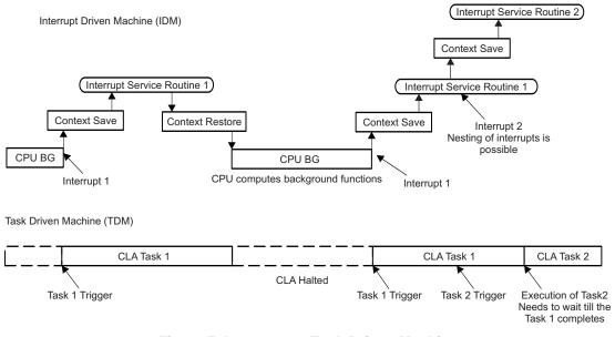
Figure 5. Interrupt vs Task Driven Machine
