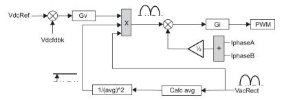
Figure 9. Digital Control Algorithm of Interleaved PFC Stage
