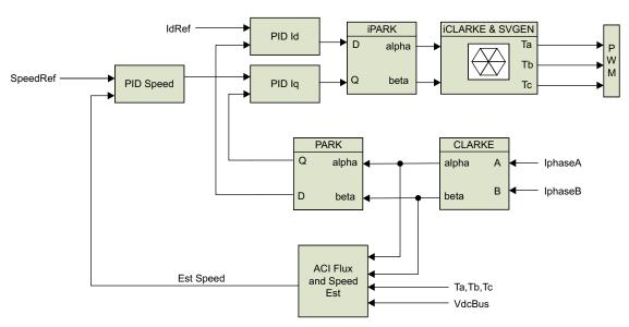
Figure 8. FOC of AC Induction Motor
