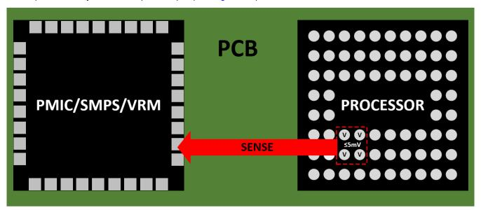
Figure 4-3. Sense Line Placement
