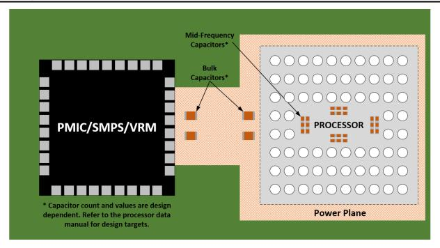
Figure 5-3. Example Capacitor Placement
