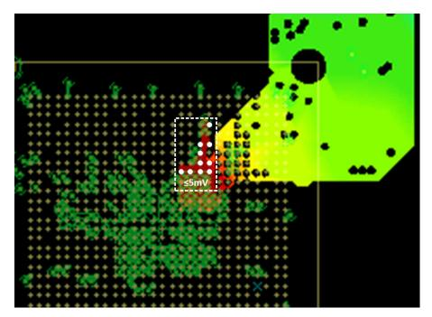
Figure 4-4. Allowable Power Input Voltage Difference
