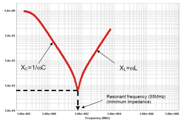
Figure 3-2. Typical Impedance Profile of a Capacitor
