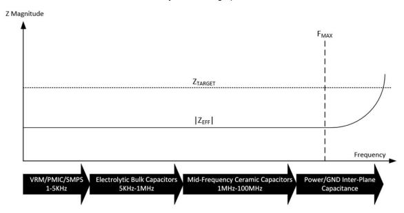
Figure 5-2. Decoupling Frequency Range of PCB Components
