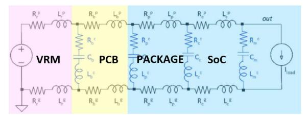
Figure 5-1. Components of a Typical Power Distribution Network (PDN)
