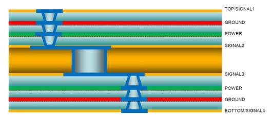
Figure 2-2. Example Stack-Up Utilizing High-Density Interconnect Vias
