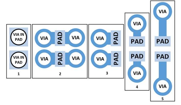
Figure 3-4. Capacitor Mounting Geometries
