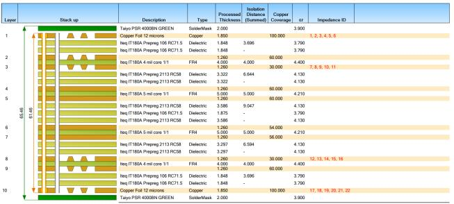
Copper Thickness = 13.779 | Dielectric Thickness = 47.677 | Solder Mask Thickness = 4.000 | Stack Up Thickness = 61.456 | Stack Up Thickness with Soldermask = 65.456
