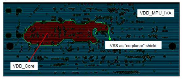
Figure 3-3. Example of "Co-Planar' Shielding of Power Net Using Ground Guard-Band
