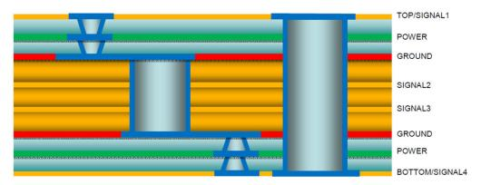
Figure 2-3. Example Stack-Up Utilizing Plated-Through-Hole (PTH) Vias
