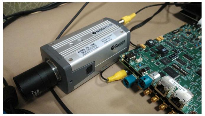
Figure 3. analog camera via TVP5158
