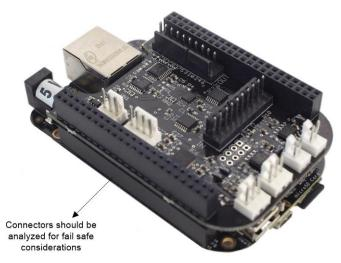
Figure 9. Multi PCB System Design
