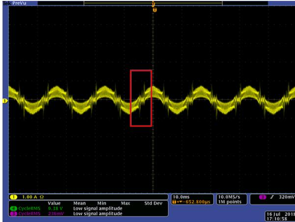
Figure 7-1. 120 V Input, 380 V Output, 40W Output: High Current Distortion Near Zero Crossing Point Without Optimized ZVS (with valley skipping) and Fixed Frequency Control
