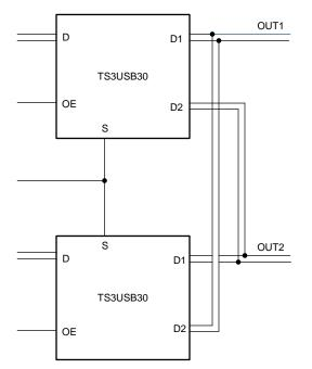
Figure 1. Function Block Diagram
