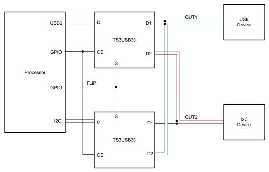
Figure 2. 2:2 Differential Cross-point Switch Schematic
