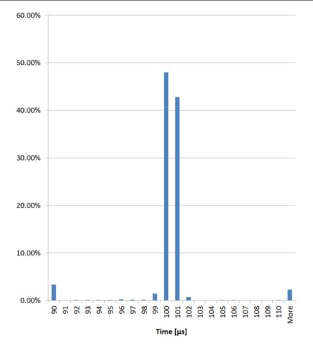
Figure 3-2. Timing Jitter with User Space Implementation
