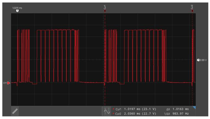
Figure 3-7. IO-link Communication with TIDA-01437 Stacklight
