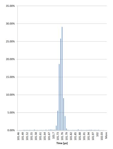
Figure 3-6. Timing Jitter with Implementation on Separate Arm Cortex-M4
