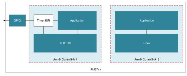
Figure 3-5. Timer on Arm Cortex M4
