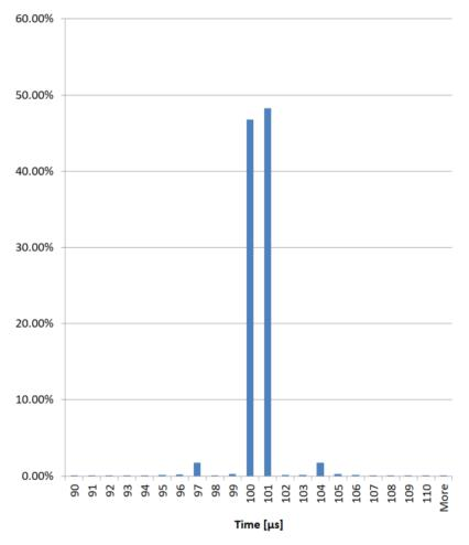
Figure 3-4. Timing Jitter with Kernel Space Implementation
