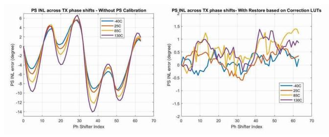
Figure 3-5. TX Phase Shifter Accuracy in the AWR22431, 2
