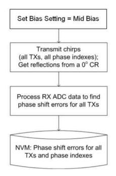
Figure A-3. Measuring TX Phase Shifter Errors at Customer Factory
