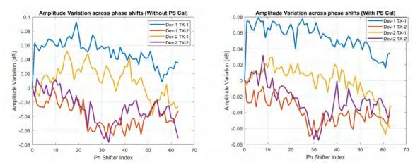
Figure 3-7. Amplitude Variation Across Phase Shifter Settings at 25C1
