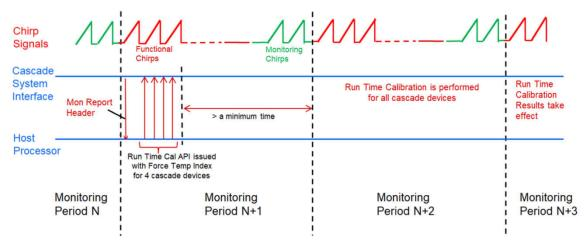
Figure 3-2. AWR2243 RunTime Cal Temp Index Forcing Timing Diagram
