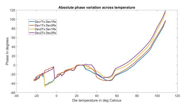
Figure 4-1. Absolute Phase Variation with Independent, Autonomous Periodic Run Time Calibrations in the Devices
