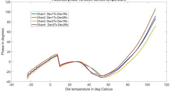
Figure 4-2. Absolute Phase Variation with External Triggering of Calibration Updates1
