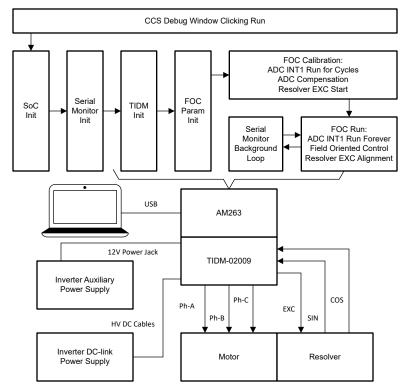
Figure 1-2. Traction Inverter System Diagram
