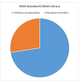
Figure 2-1. AM26x Software Computation vs Hardware Interface for FOC Loop With Standard C lib
