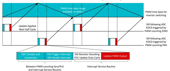
Figure 3-2. Sample ADC in First Half of Cycle 0 and Update PWM in Second Half of Cycle 0
