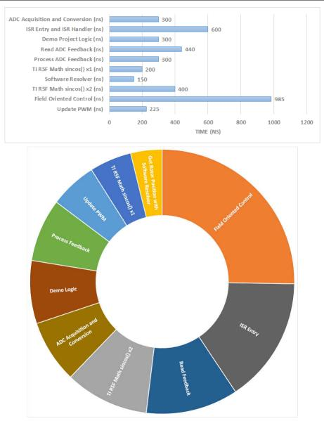
Figure 2-4. AM26x Time Consumption Breakdown for FOC Loop With TI R5F lib
