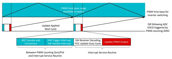
Figure 3-1. Sample ADC in Cycle 0 and Update PWM in Cycle 1
