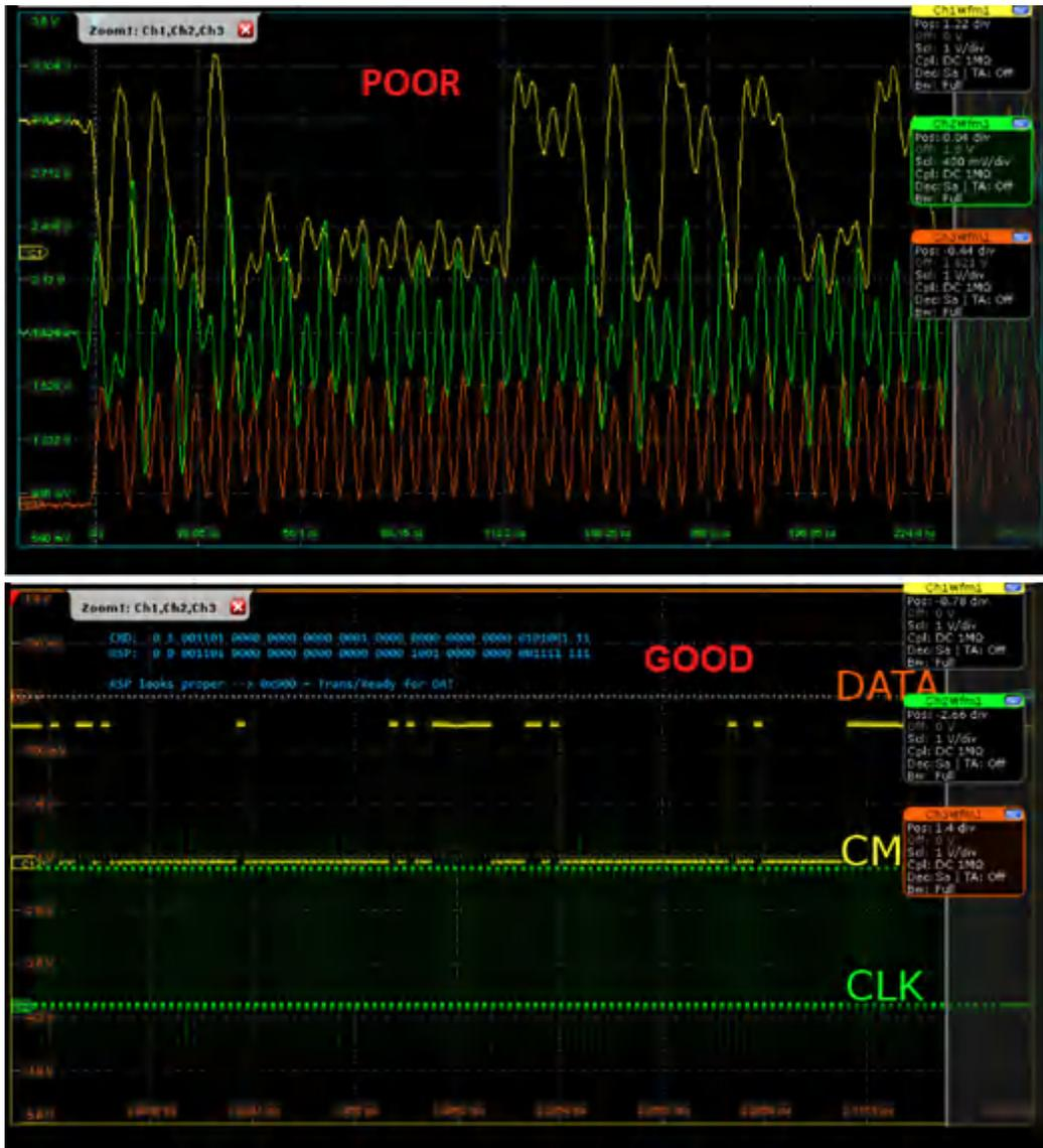
Figure 5-1. Poor Signal Integrity vs Good Signal Integrity on DATA, CMD, and CLK
