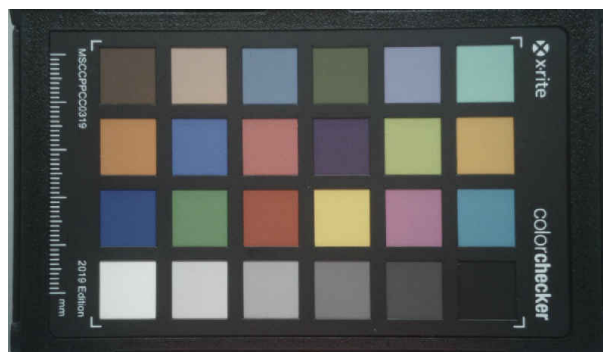
Figure 6-16. Image After Auto White Balance Tuning
