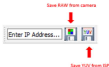
Figure 6-7. Live Capture Feature of DCC Tuning Tool
