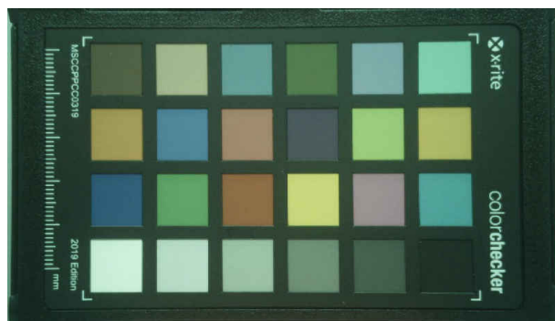
Figure 6-15. Image Before Auto White Balance Tuning
