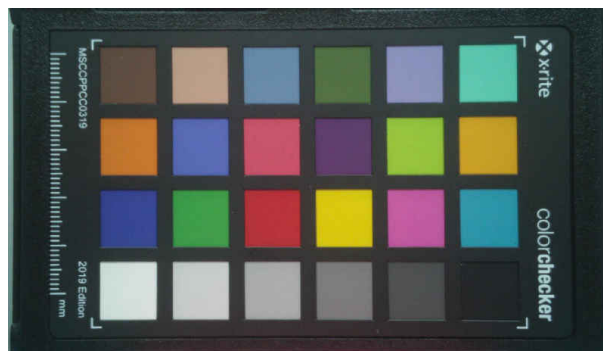
Figure 6-20. Image After Color Correction Tuning
