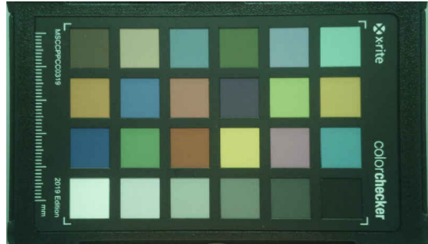
Figure 6-6. Image After Black Level Subtraction
