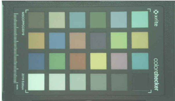
Figure 6-5. Image Before Black Level Subtraction
