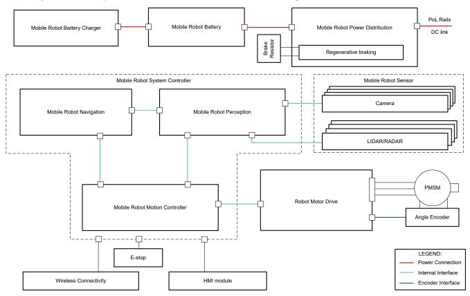
Figure 2-1. Simplified Mobile Robot Block Diagram
