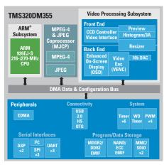
TMS320DM355 processor block diagram
