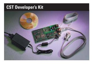
the TMS320C54CST DSP and 14 on-chip algorithms; external Flash, SRAM, JTAG connector and daughter card connection; RS-232 cable, RJ-11 phone line and power supply. A TI reference design features all schematic and layout guidelines, the bill of materials list and all documentation including a CD-ROM with board manual, quick start guide and a C54CST DSP overview.
