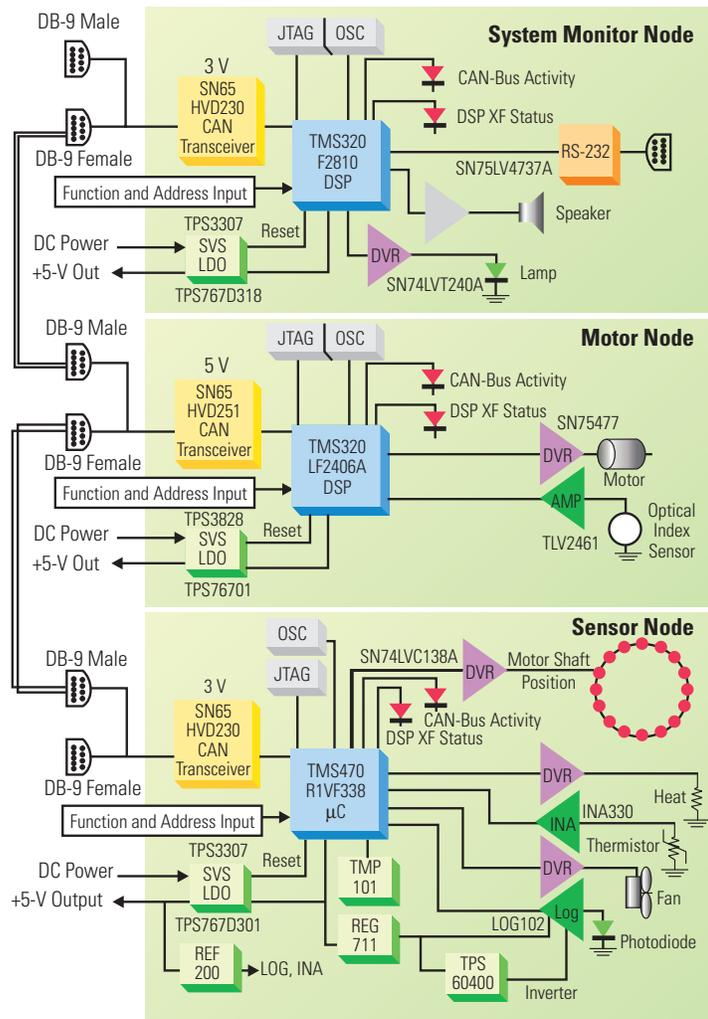
Figure 2: CAN-Bus Platform Block Diagram
