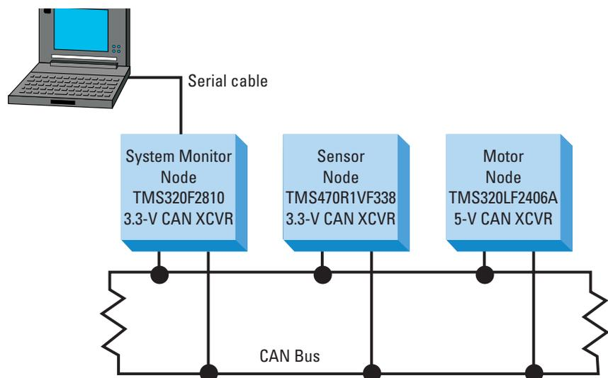
Figure 1. CAN-bus nodes.
