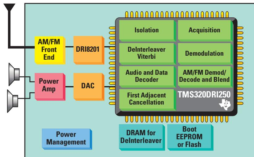
The TMS320DRI250 implements the baseband processing for both HD Radio and AM/FM on a single device. The DRI8201 samples and downconverts the intermediate frequency (IF) from the AM/FM front end.
