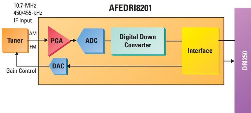
*ADC and DDC integrated to provide precision AM/FM and HD Radio digitization.*
