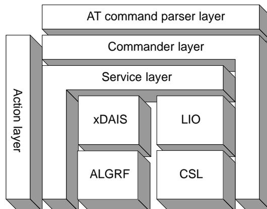
CST Framework has two alternative top layers and therefore, two alternative top-level interfaces.
