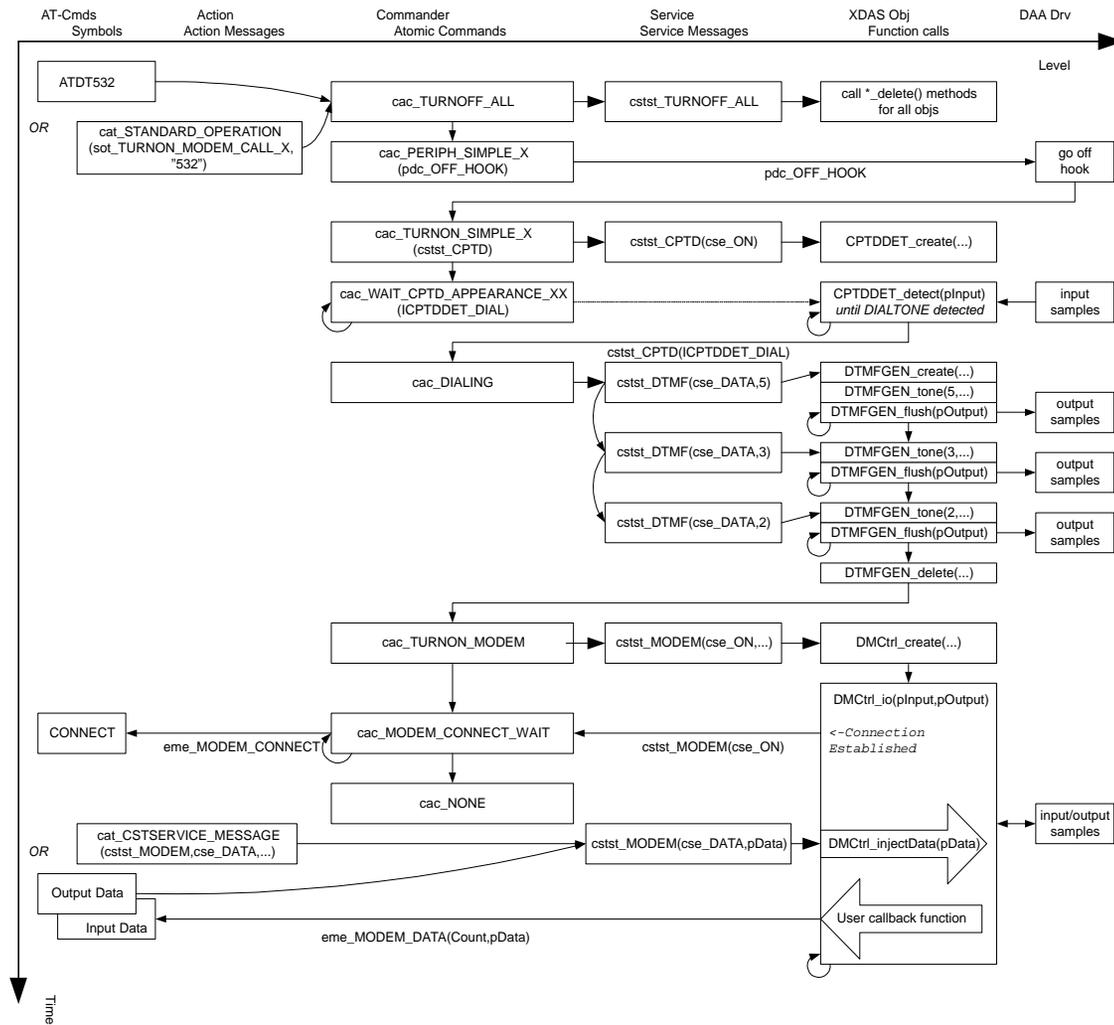
Once again, either AT commands (usually, in Chipset mode) or CST Actions (in Flex mode) are used. These are the two mutually exclusive ways to control the CST solution.
