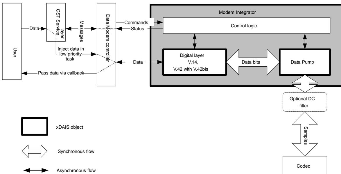
As it has been mentioned, the modem passes the decoded data through a callback function. Besides this data callback function, there are two other (optional) callback functions to be implemented by user.
