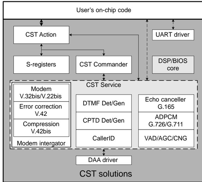
The action interface is based on interfaces of sublayers without essential modifications. The action interface allows the user to begin integration into the CST Framework.
