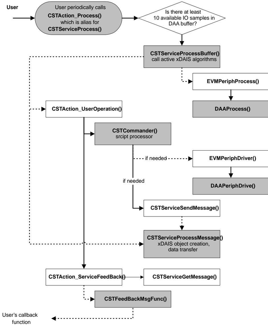
The key functions are painted in gray. Dotted arrows represent dynamic function calls, e.g. the functions are called through the `CSTFxnS` pointers. The Action, Commander, Service control layers, high-level DAA driver and the peripheral driver are presented by the following functions:
