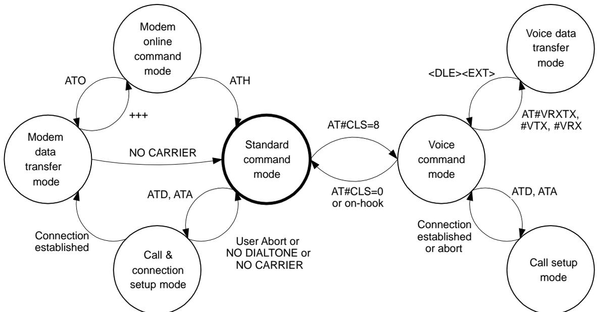
After initialization, AT parser is in standard command mode. If `ATD` or `ATA` command is issued, it will start dialing, and will be in call and connection setup mode until connection is established, and then will move to modem data trans-
