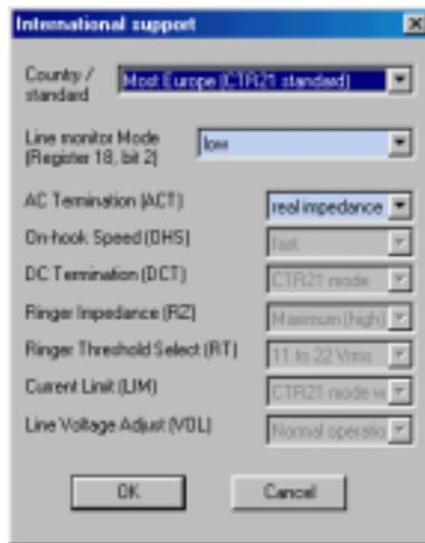
Line monitor mode controls bit 2 of DAA register 18 (S register 118). If it selected as “high”, this bit is set to 1, otherwise – to 0. This bit influences DAA functionality in conjunction with several other bits, detailed description of this is given in *TMS320C54CST Client Side Telephony DSP. Data Manual. Texas Instruments (SPRS187)*. For the most part, this bit is used to control on-hook current line monitor – high or low.
