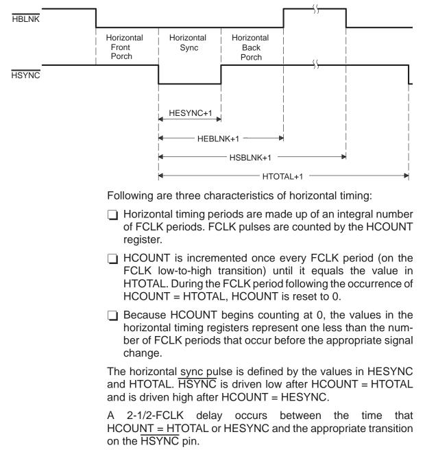
Figure 4–2. Horizontal Timing Signals
