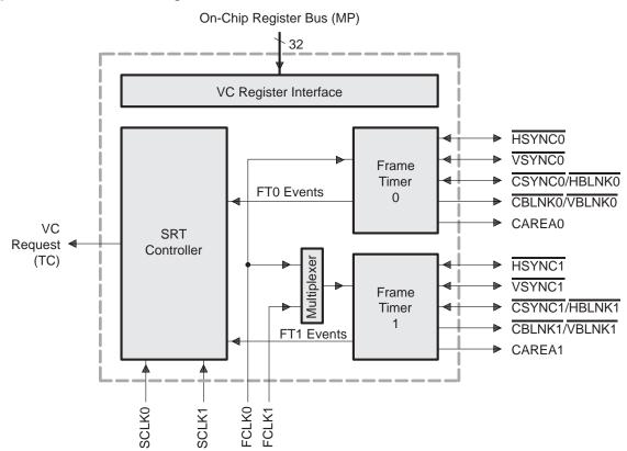
Figure 1–2. VC Block Diagram
