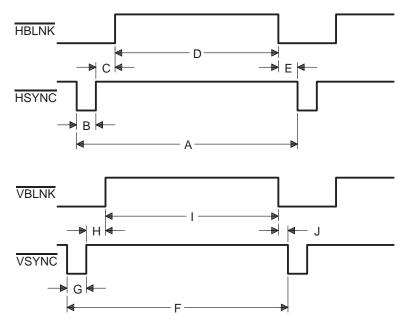
Table A–1. Typical Noninterlaced Monitor Timing
