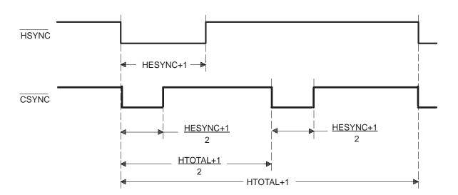
Broadcast-quality composite-video standards, such as NTSC and PAL, require that equalization pulses are exactly half the duration of horizontal-sync pulses. Since HCOUNT counts from 0, you should set HESYNC to an odd value so that horizontal sync is an even number of FCLK cycles in length and, thus, evenly divisible by 2. HTOTAL should also be programmed to an odd value so that HTOTAL/2 occurs exactly midway through each horizontal line.
