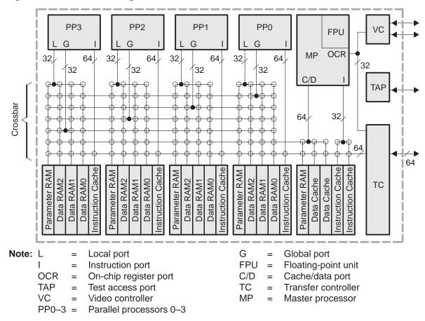
Figure 1–1. MVP Block Diagram
