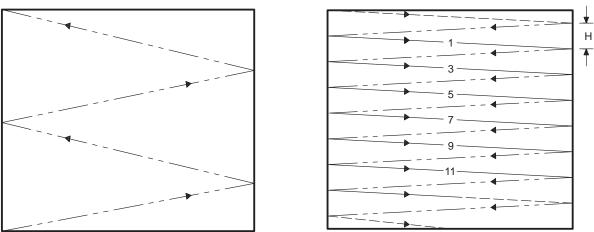
Figure 4–12 (a) shows the vertical retrace that precedes the odd field. It consists of an integral number of horizontal halflines.
