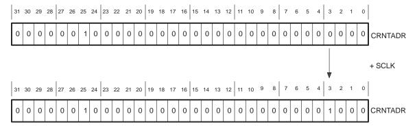
Once the value in the CRNTADR register has reached 0x0200 03F8, the next SCLK causes an overflow in the bits corresponding to the SAMMASK register, and an overflow event is generated, as Figure 5–3 shows.
