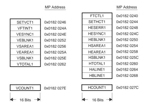
As Figure 1–4 and Figure 1–5 illustrate, horizontal timing registers are located at even halfword addresses. Their vertical counterparts are located at odd halfword addresses.
