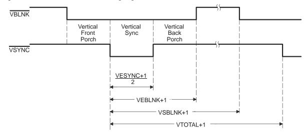
Following are three features of interlaced vertical timing signals:
