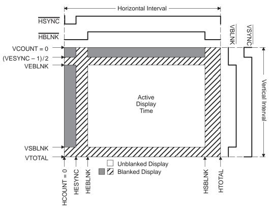
The timing of the horizontal and vertical sync and blanking pulses depends on the display that you are using. The relationship between the sync and blanking pulses shown in Figure A–1 defines what are known as the **porches** in video timing. The porches are shown in Figure A–2.
