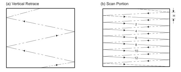
Figure 4–13 (a) shows the vertical retrace that precedes the even field. It consists of an integral number of horizontal halflines.
