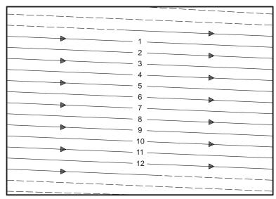
Figure 4–14. Scan Pattern for Interlaced Monitors—Both Fields
