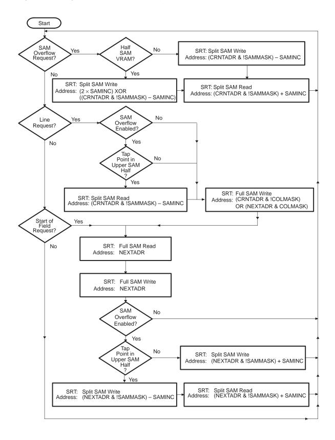
Figure 5–7. Merge Capture Mode SRT Sequence
