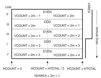
In general, VEAREA must be set to whichever value of VCOUNT is common to the last even and odd lines before VAREA is required to be inactive. For the NTSC standard, VCOUNT is always **even** at the end of even lines and **odd** at the end of odd lines. For the PAL standard, the opposite is true; VCOUNT is always **odd** at the end of even lines and **even** at the end of odd lines. VEAREA programming for the PAL standard is shown in Figure 4–21.
