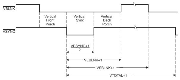
Following are three characteristics of the noninterlaced vertical timing signals:
