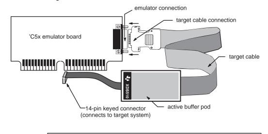
Figure 2–3. Emulator Target Cable and Board
