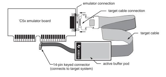
Figure 1–3. Connecting the Target Cable to the 'C5x Emulator Board
