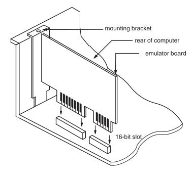
Step 5: Tighten down the mounting bracket.
