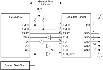
There are two benefits to having the target system generate the test clock:
