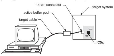
Figure 2–5 shows how you connect the emulator and target cable to your target system. In most cases, the target system will be a 'C5x board of your own design.
