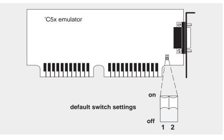
Switches are shipped in the default settings shown here and are listed in Table 2–1. If you use an I/O space that differs from the default, change the switch settings. Table 2–1 shows alternate settings.
