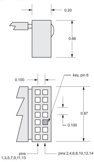
Figure 3–7. 14-Pin Connector Dimensions
