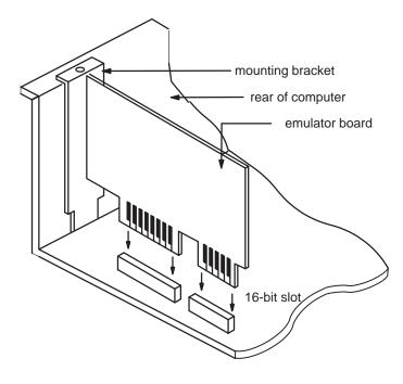
**Step 5:** Tighten down the mounting bracket.
