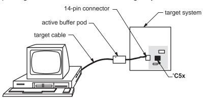
Figure 1–5 shows how you connect the emulator and target cable to your target system. In most cases, the target system will be a 'C5x board of your own design.
