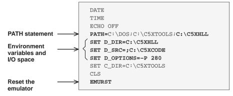
(a) Sample autoexec.bat file to use with the debugger and emulator
