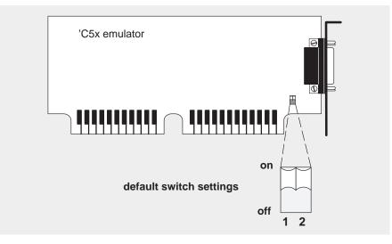
Switches are shipped in the default settings shown here and are listed in Table 1–1. If you use an I/O space that differs from the default, change the switch settings. Table 1–1 also shows alternate settings.
