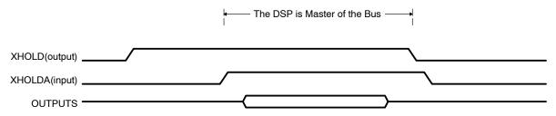
When the internal bus arbiter is disabled and the XBUS master transfer is initiated by writing to the START bits of XBHC, the DSP asserts its XHOLD request. If the host initiates a transfer to the DSP instead of granting the DSP access to the XBUS, the DSP drops its XHOLD request as shown in Figure 23.
