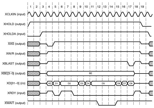
Note: XWAIT is an output only signal in synchronous host port mode.
