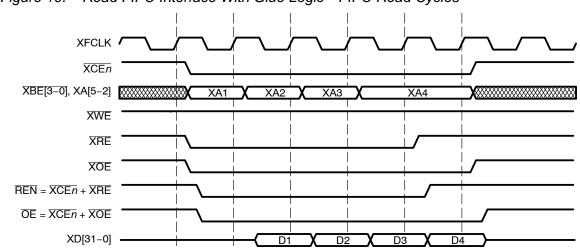
Figure 10. Read FIFO Interface With Glue Logic—FIFO Read Cycles
