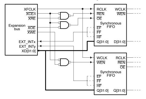
Figure 7. Read and Write FIFO Interface With Glue Logic—FIFO Write Cycles
