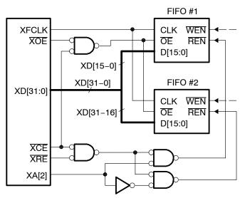
Table 4. Addressing Scheme—Expansion Bus Interfaced to Two 16-Bit FIFOs
