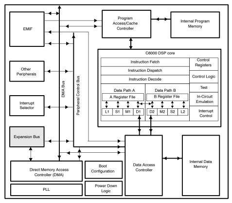
Figure 2. TMS320C62x DSP Block Diagram
