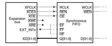
Figure 9. Read FIFO Interface With Glueless Logic—FIFO Read Cycles
