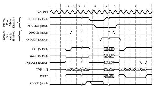
The timing diagram in Figure 17 can be referenced for a visual description of the steps involved in release of the XBUS ownership as initiated by the XBOFF signal. Figure 17 shows the backoff condition for both internal bus arbiter enabled and internal bus arbiter disabled. The step-by-step description of the events marked above the waveforms in Figure 17:
