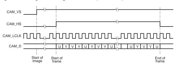
Figure 3. Timing Chart of Image Data Transfer (POLCLK = 1)
