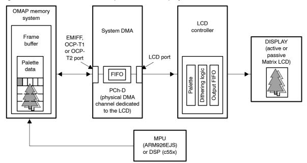
Figure 2. Data Flow from Microprocessor to Display
