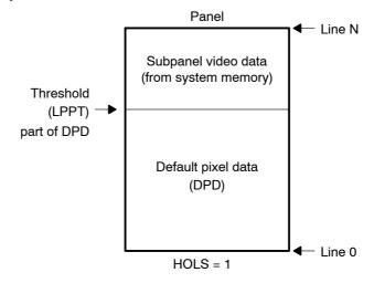
When HOLS = 0, the beginning of the screen is filled with DPD value until the LPPT excluded. From the LPPT line number, the rest of the screen (below LPPT) displays the image from system memory.
