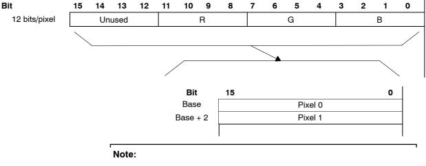
Unused [15..12] bits are filled with zeroes in TFT mode.
