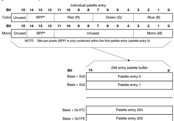
Figure 5. 256-Entry Palette/Buffer Format (8 BPP)
