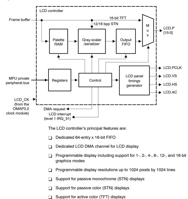
Figure 1. LCD Controller
