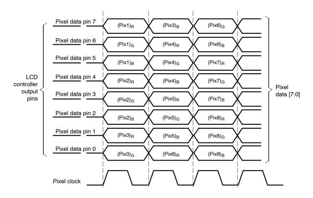
After the pixel clock toggles three times, the situation returns to its initial state. At the fourth clock cycle, the figure becomes identical to itself, i.e., the number of pixels displayed is an integer.
