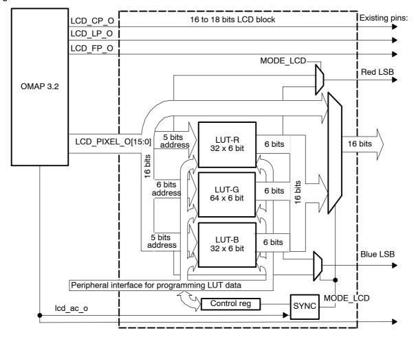
Figure 39. 16-Bit to 18-Bit LCD Data Block
