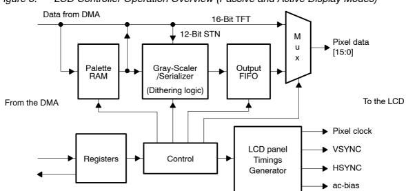
Figure 3 illustrates the LCD controller logic.
