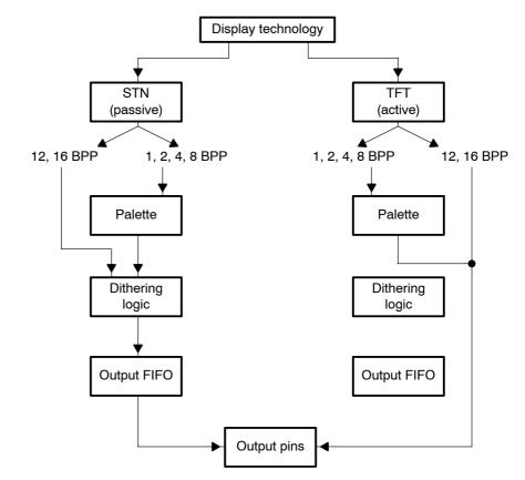
Figure 14. LCD Controller Data Paths
