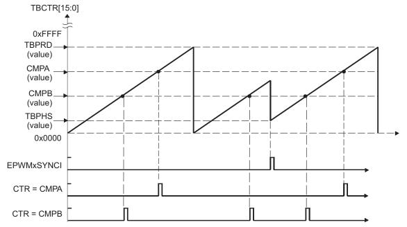
Figure 2-13. Counter-Compare Event Waveforms in Up-Count Mode
