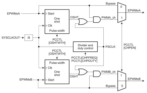
Figure 2-31. PWM-Chopper Submodule Operational Details
