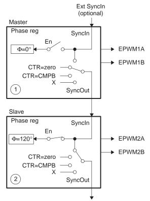
Figure 3-12 shows the associated timing waveforms for this configuration. Here, TBPRD = 600 for both master and slave. For the slave, TBPHS = 200 (i.e., 200/600 X  $360^\circ = 120^\circ$ ). Whenever the master generates a Syncln pulse (CTR = PRD), the value of TBPHS = 200 is loaded into the slave TBCTR register so the slave time-base is always leading the master's time-base by 120°.
