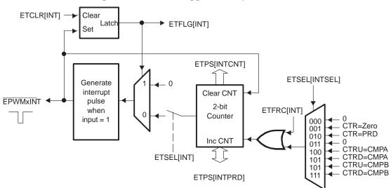
Figure 2-41. Event-Trigger Interrupt Generator
