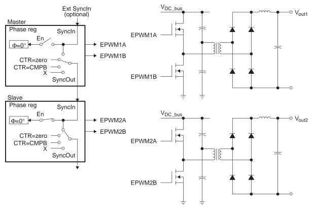
Figure 3-7. Control of Two Half-H Bridge Stages (F<sub>PWM2</sub> = N x F<sub>PWM1</sub>)
