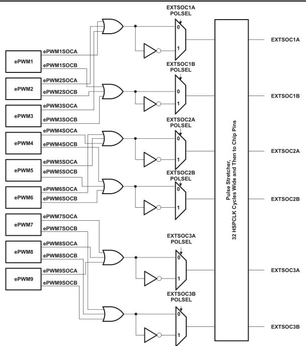
The event-trigger submodule monitors various event conditions (the left side inputs to event-trigger submodule shown in Figure 2-40) and can be configured to prescale these events before issuing an Interrupt request or an ADC start of conversion. The event-trigger prescaling logic can issue Interrupt requests and ADC start of conversion at:
