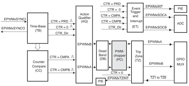
The PWM-chopper submodule allows a high-frequency carrier signal to modulate the PWM waveform generated by the action-qualifier and dead-band submodules. This capability is important if you need pulse transformer-based gate drivers to control the power switching elements.
