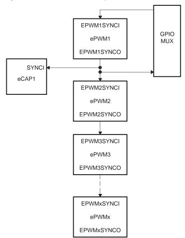
Figure 2-4. Time-Base Counter Synchronization Scheme 1
