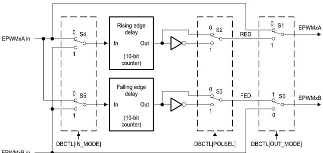
Figure 2-28. Configuration Options for the Dead-Band Submodule
