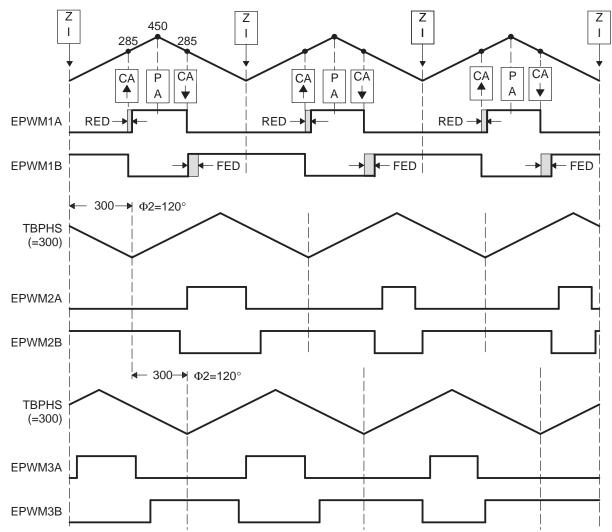
Figure 3-14. 3-Phase Interleaved DC/DC Converter Waveforms for Figure 3-13
