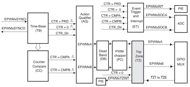
Each ePWM module is connected to six  $\overline{TZn}$  signals ( $\overline{TZ1}$  to  $\overline{TZ6}$ ) that are sourced from the GPIO MUX. These signals indicate external fault or trip conditions, and the ePWM outputs can be programmed to respond accordingly when faults occur.
