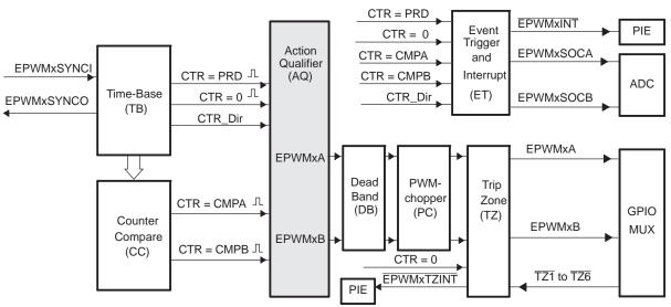
The action-qualifier submodule has the most important role in waveform construction and PWM generation. It decides which events are converted into various action types, thereby producing the required switched waveforms at the EPWMxA and EPWMxB outputs.
