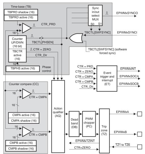
Figure 1-3. ePWM Submodules and Critical Internal Signal Interconnects
