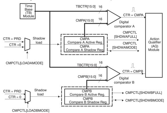
Figure 2-12. Detailed View of the Counter-Compare Submodule
