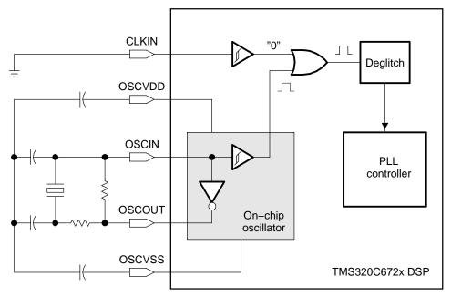
Figure A-2. OSCIN Pin Used as Reference Clock Source
