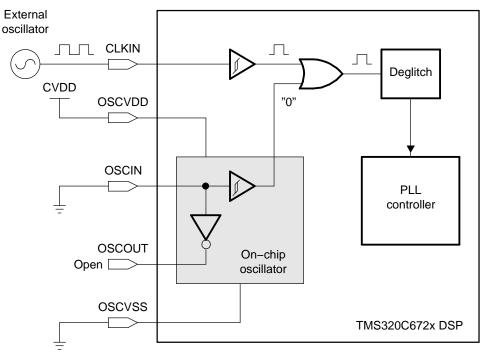
Figure A-1. CLKIN Pin Used as Reference Clock Source
