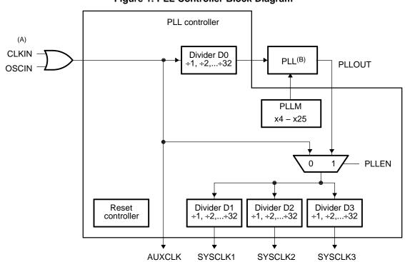
Figure 1. PLL Controller Block Diagram
