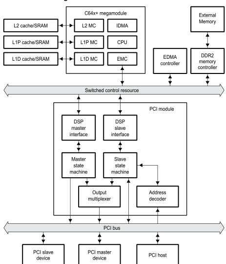
Figure 6. PCI to External PCI Device
