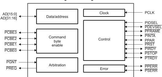
Figure 2. PCI Signals
