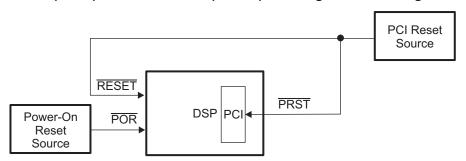
Figure 5. Independent External Power-On Reset (POR), Warm Reset (RESET), and PCI Reset (PRST)
