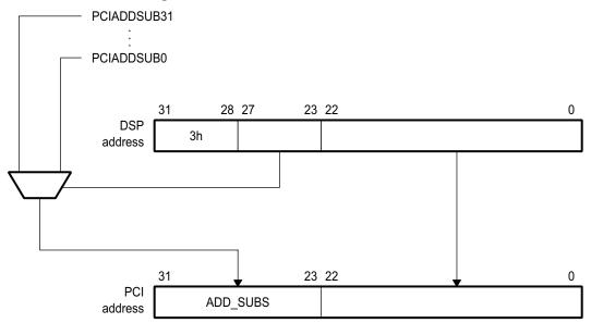
Figure 11. DSP-to-PCI Address Translation
