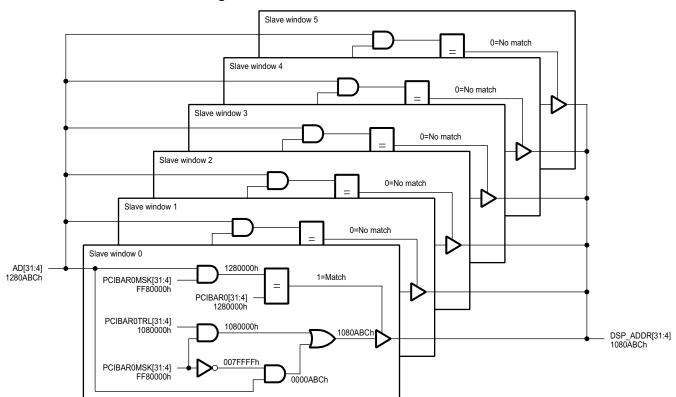
Figure 8. PCI-to-DSP Address Translation
