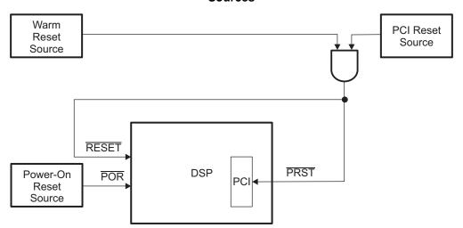
In Figure 4 and Figure 5, a device-level global reset resets the DSP and the PCI module only; other devices on the PCI bus will not be reset. To avoid interrupting any ongoing PCI transactions to/from the DSP, the PCI module should be "disconnected" from the PCI system.
