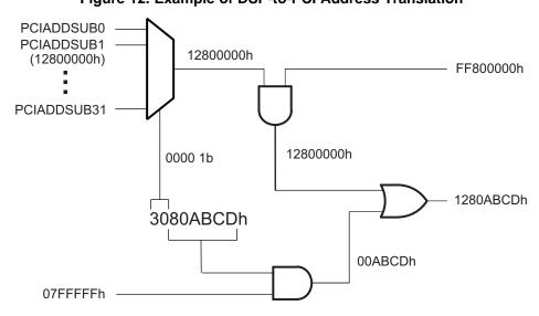
Figure 12. Example of DSP-to-PCI Address Translation
