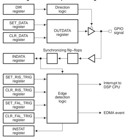
Figure 1. GPIO Peripheral Block Diagram
